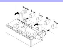
Connect it directly to the measurement jacks with the label side facing up, and fix it with the levers on the left and right sides.
