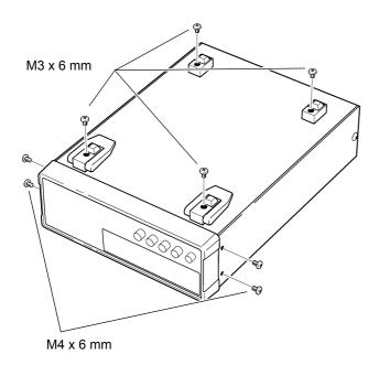
Remove the feet from the bottom of the instrument, and the screws from the sides (four near the front).
