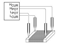
Figure 11. Four-Terminal Measurement
