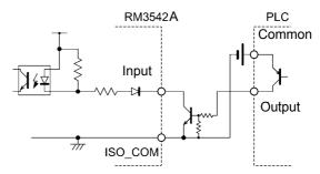
PLC Output (Source Output) Connections
