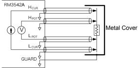
Figure 2. For High-Resistance Measurements
