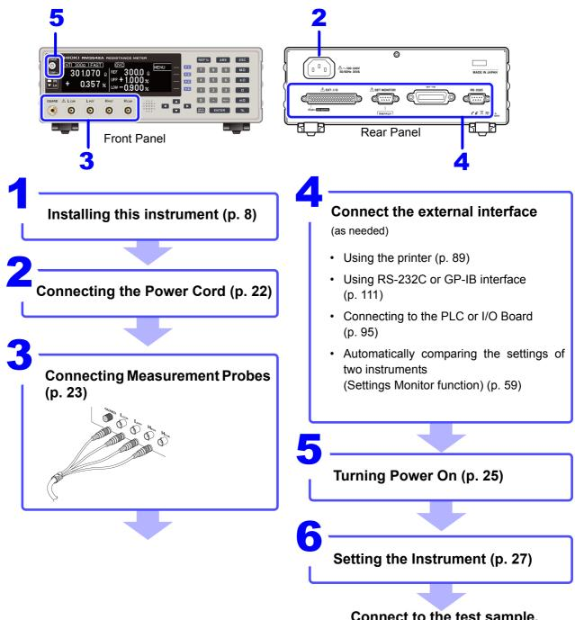
Connect to the test sample.
