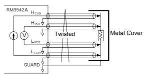
Figure 3. For Low-Power Resistance Measurements
