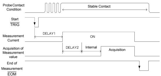
\* Internal delay is provided to suit purely resistive (non-reactive) measuring objects, and is different for each measurement range.
