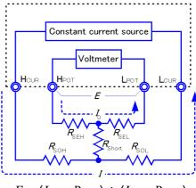
$$E = (I_0 \times R_{SEL}) + (I_0 \times R_{SEH})$$
