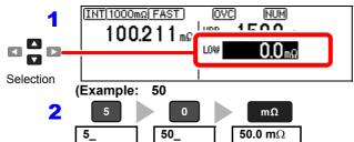
Press the units key to accept the setting and move the cursor to the upper threshold.
