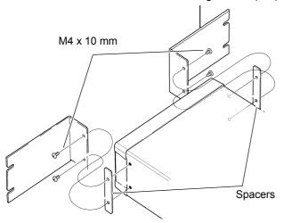
Insert the spacers on both sides of the instrument, attach the Rack Mounting Blackets with the M4 x 10 mm screws.
