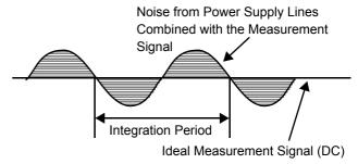
Figure 1. Effect of Noise from Power Supply Lines
