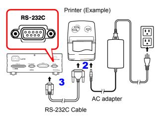
Confirm that the instrument and the printer are turned off.
