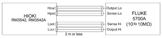
Calibration using Fluke 5700A at 10  $\Omega$  to 10  $\text{M}\Omega$
