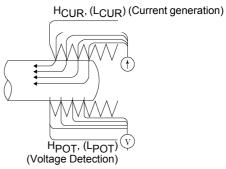
Figure 5. Measurement with Model 9140 4-Terminal Probe
