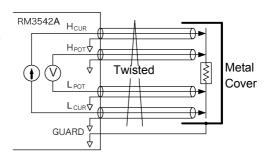
Figure 9. Wiring to Minimize Noise Ingress
