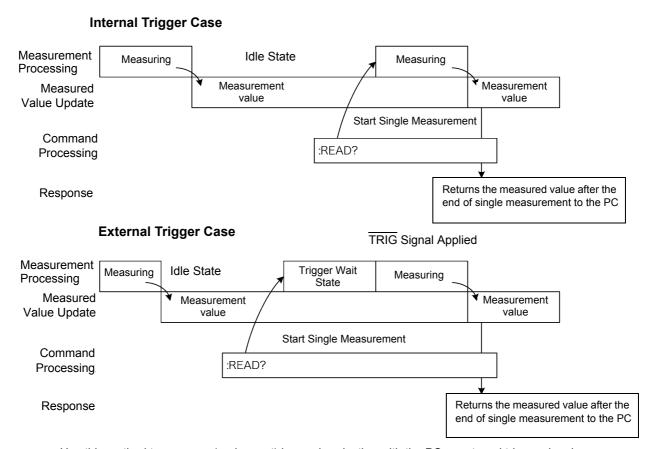
Use this method to measure (and export) in synchronization with the PC or external trigger signal. Measurement time can be minimized.
