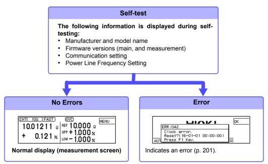
When the power is turned on, the same setting as when the power was last turned off appears (backup function).
