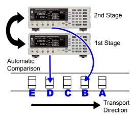
Connect the SET MONITOR connectors of the two instruments using a Hioki 9637 RS-232C cable.
