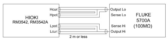
Calibration using Fluke 5700A at 100  $M\Omega$
