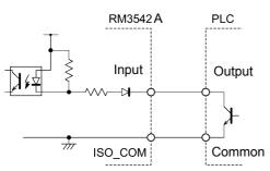
PLC Output (Sink Output) Connections
