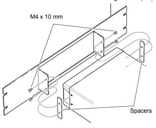
When installing in a rack, support it by a stand or other commercially available items.
