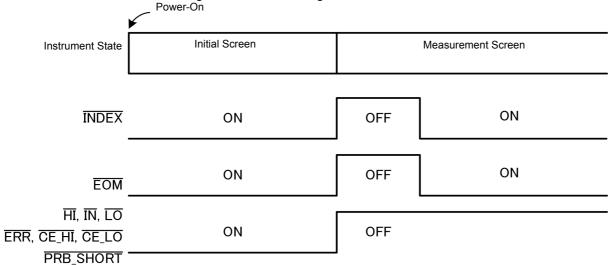
This shows the operations when the trigger source is set to an external trigger, [EXT].
