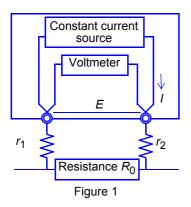
Measurement current I flows through the test object resistance  $R_0$  as well as lead resistances  $r_1$  and  $r_2$ . Therefore, voltage measured will be given by  $E = I(r_1+R_0+r_2)$  which includes lead resistances  $r_1$  and  $r_2$ .
