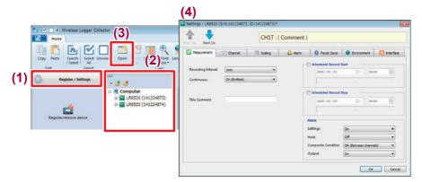
5 Send the measurement conditions to the instrument.
