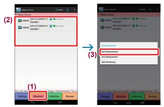
6 Collect measurement data using Wireless Logger Collector.
