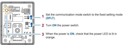
If the power LED is not lit in orange, the setting of the communication mode switch may be incorrect or the instrument may malfunction. If the instrument malfunctions, stop the setting and send the instrument for repair.
