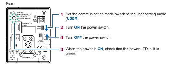
If the power LED is not lit in green, the setting of the communication mode switch may be incorrect or the instrument may malfunction. If the instrument malfunctions, stop the settings and send the instrument for repair.
