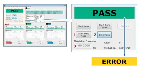
This display is shown when the measurement cannot be performed correctly. (p.78)
