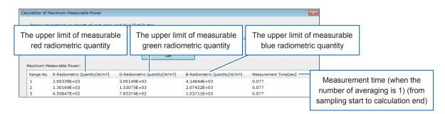
The upper limit of measurable radiometric quantity may exceed the maximum input. However, the radiometric quantity to be input to the instrument should not exceed the maximum input.
