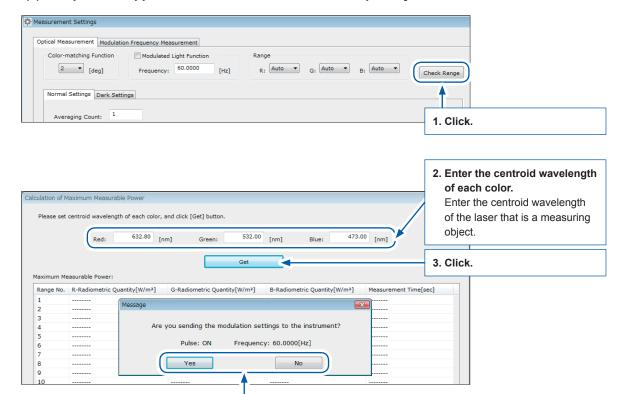
4. Check the sending of the modulated light function and modulation frequency setting.
