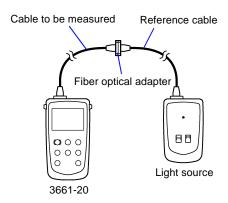
4. The optical loss of the cable to be measured appears on the LCD.
