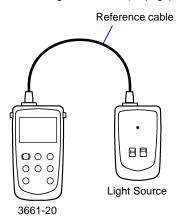
Press DISPLAY POWER/LOSS key to select optical power measurement mode.
