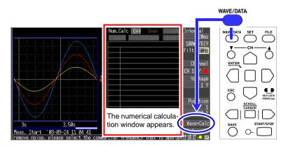
2 Enable [Num.Calc] (set to On), and set up to four calculation types (1 to 4).
