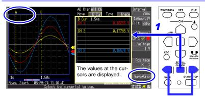
2 Press these keys to move the cursor on the displayed waveform.
