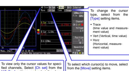
fied channels, Select [Ch set] from the [AB Crsr] settings, and select the channels for which to display cursor values.
