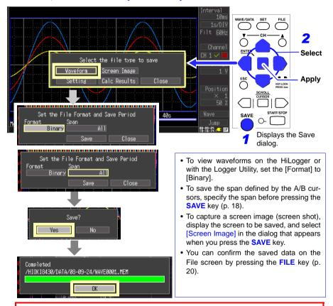
For long-term measurement, set the Auto-Save setting to [Waveform(realtime)] (p. 9). When [Cont] is enabled, data recording is limited to the size of the HiLogger's internal memory.
