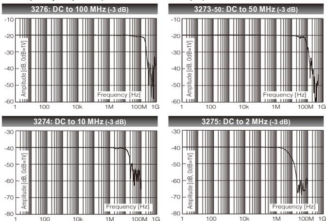
Note: use the Power Supply 3269/3272 for general measurements or when power is not available from the Memory HiCorder. When performing continuous measurements, be aware of offset voltage drift.
