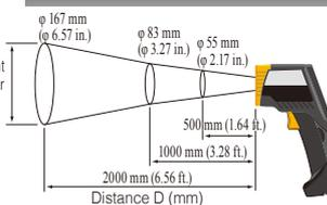
FT3701-20 Measurement distance and field diameter
