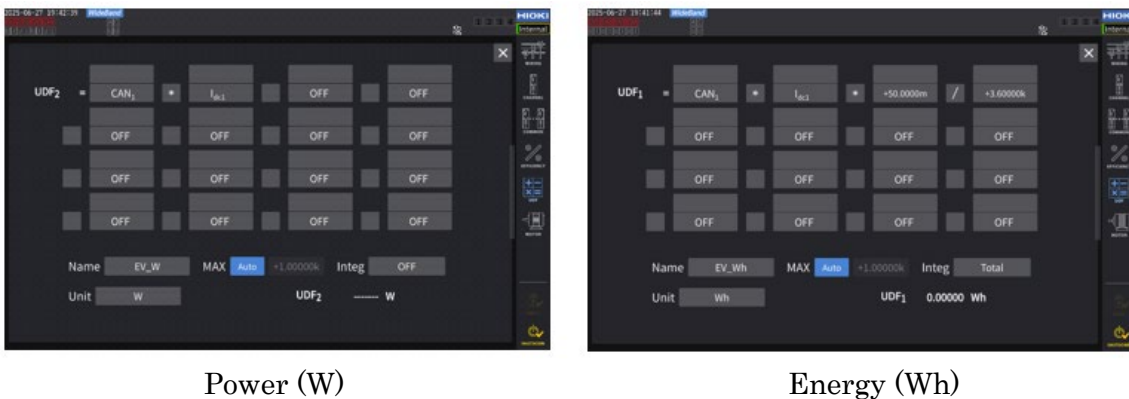
Fig. 9. Calculation Example Using CAN Voltage and Measured Current
