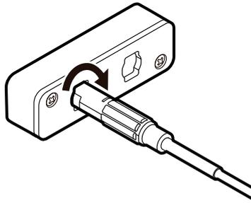
**4 Check to ensure that the unterminated lead cable connector cannot be removed.**
