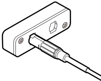
**3 Turn the unterminated lead cable connector 90 degrees and lock it.**
