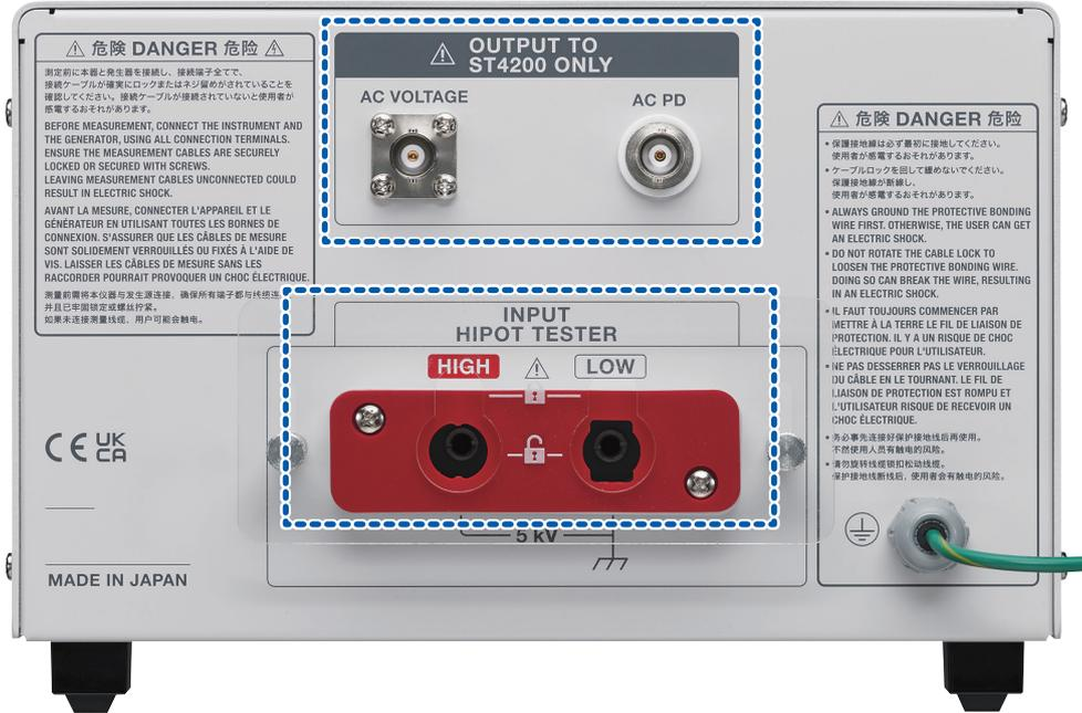
Select the connectors on the instrument side and the connection cables depending on the instrument being connected.
