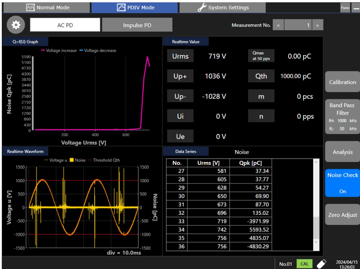
When PD occurs, the value of **Qpk** rapidly increases. Decide on a suitable value for the threshold value to separate noise and PD from the value of **Qpk** before and after this rapid increase.
