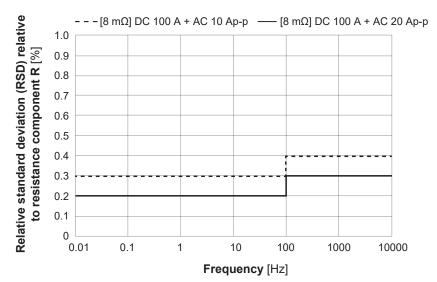
Relative standard deviation of measured resistance value when measuring resistive load (R = 8 m $\Omega$ , 100 A DC)
