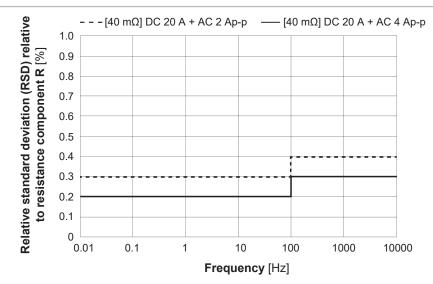
Relative standard deviation of measured resistance value when measuring resistive load (R = 40 m $\Omega$ , 20 A DC)
