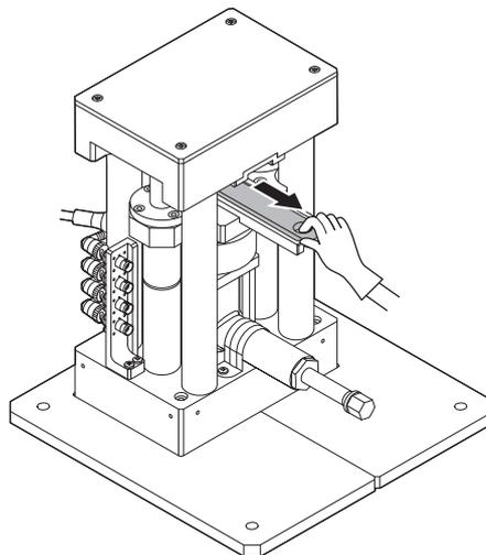
**19** Position the short-compensation block on the rail of the Press Unit.
