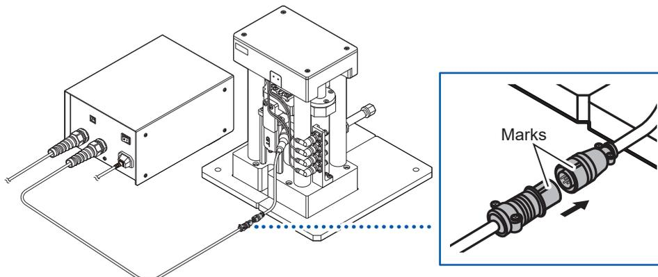
**5** Connect the displacement-sensor connector to the displacement-meter terminal of the Press Unit.
