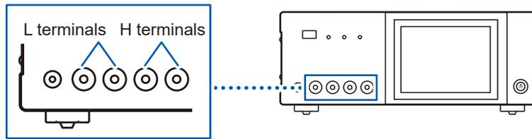
When connecting to the RM3545A, connect the red plugs to the Source A and Sense A terminals, the black plugs to the Source B and Sense B terminals, and the guard plug to the Guard terminal.
