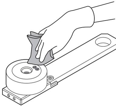
**7 Position the upper electrode of the Test Fixture onto the die, and rotate the upper electrode several times to flatten the powder in the recess.**
