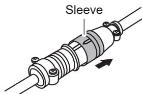
**2** Once unlocked, pull out the load-cell connector of the Sensor Unit.
