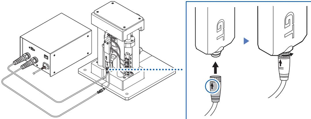
**Removing the Sensor Unit from the Press Unit**
