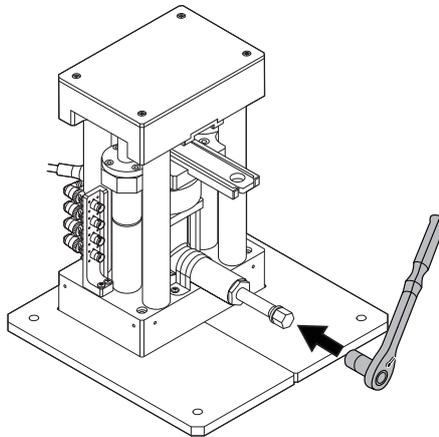
Using the switch lever of the ratchet handle can switch between two ratchet handle modes: tightening mode (clockwise) and loosening mode (counterclockwise).
