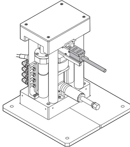
**20** Insert the short-compensation block deeply into the rail.
