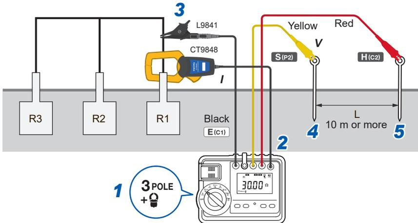
Always execute a zero adjustment before measurements. (p.82)
