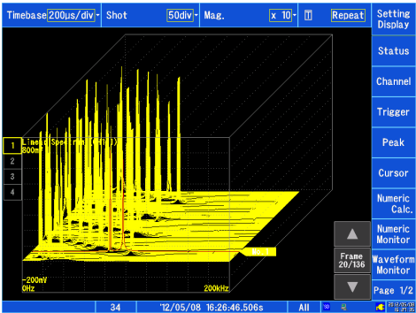
Running Spectrum (Display format: [FFT])
