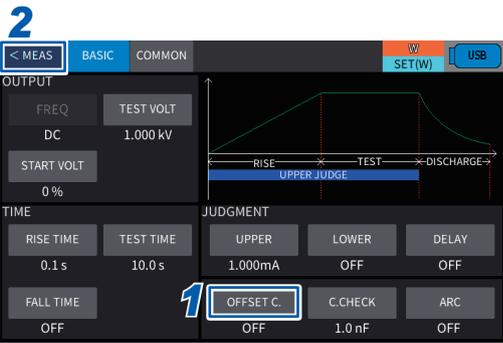
**1** On the setting screen, press [**BASIC**] > [**OFFSET C.**] to set the offset cancel function to [**ON**].
