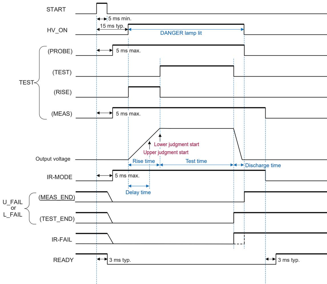
**IR test (fail judgment): With delay time setting (delay time > rinse time) and contact check (contact error)**
