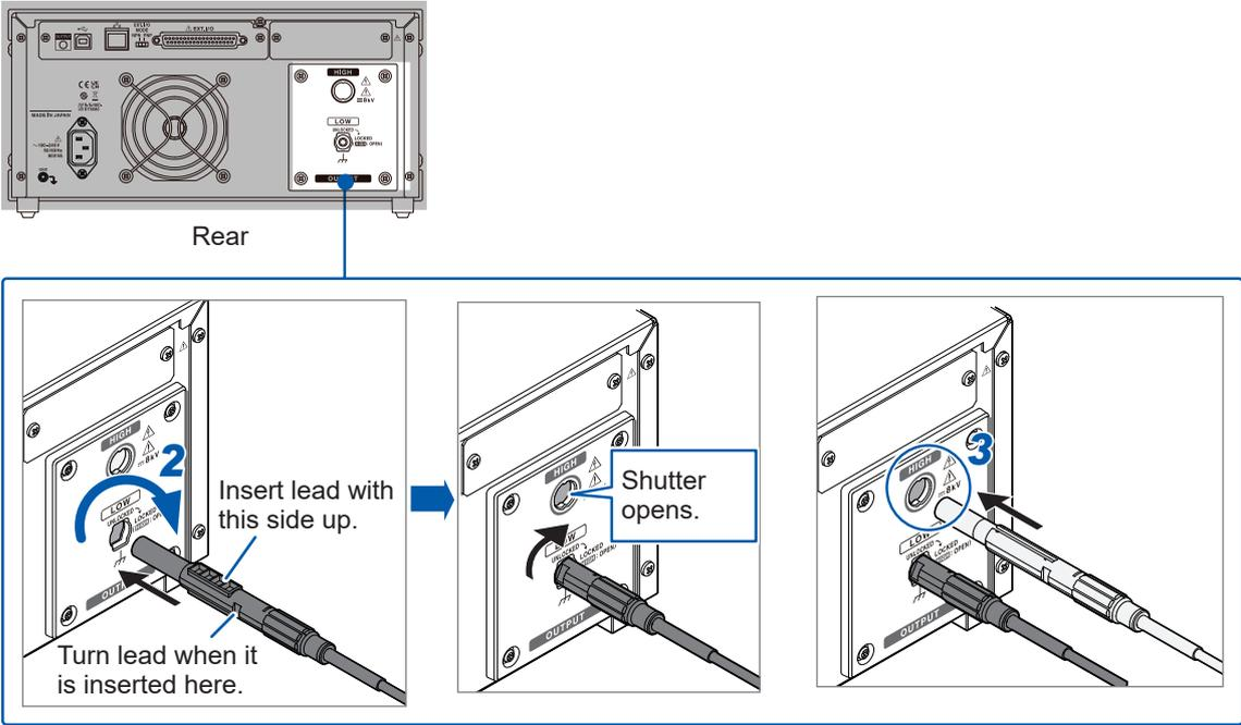
Removing the High Voltage Test Lead
