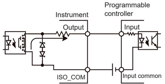
**Connection to programmable controller (positive common inputs)**
