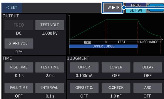
Press this button to switch the test mode.
