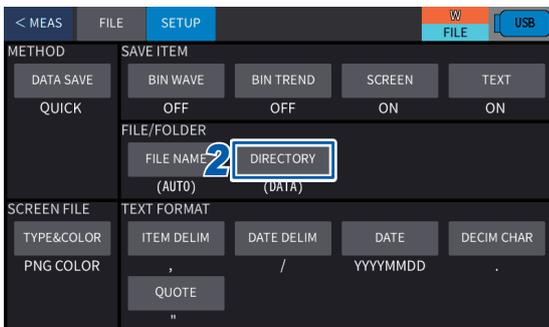
**1** Press [FILE] > [SETUP] on the measurement screen.
