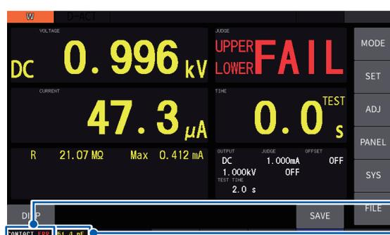
On the measurement screen, a contact check is executed at the end of the test.
