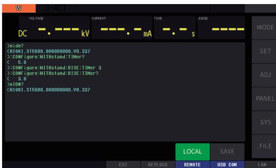
When this function is set to **[ON]**, the communication monitor is displayed on the measurement screen.
