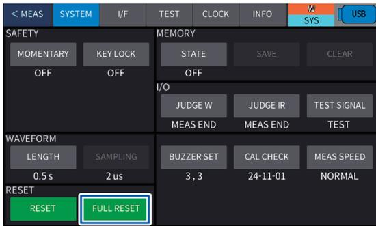
1 Press [SYSTEM] > [FULL RESET] on the measurement screen.
