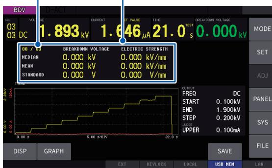
NUM + GRAPH (measured value + waveform/graph, small) display
