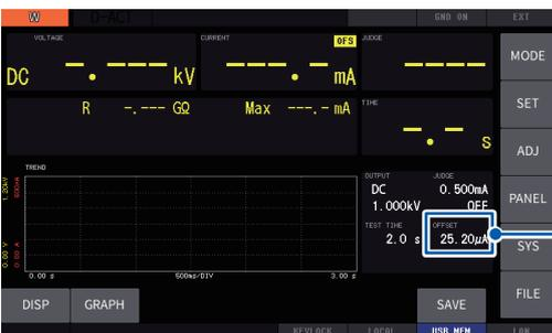
The current compensation values can also be checked on the measurement screen.
