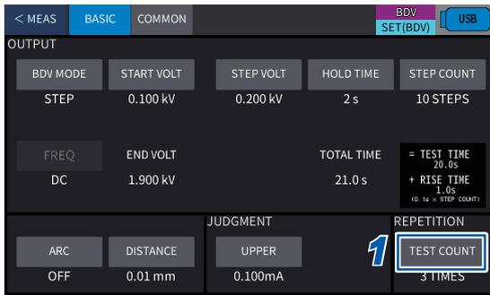
**1** Press [BASIC] > [TEST COUNT] on the setting screen.
