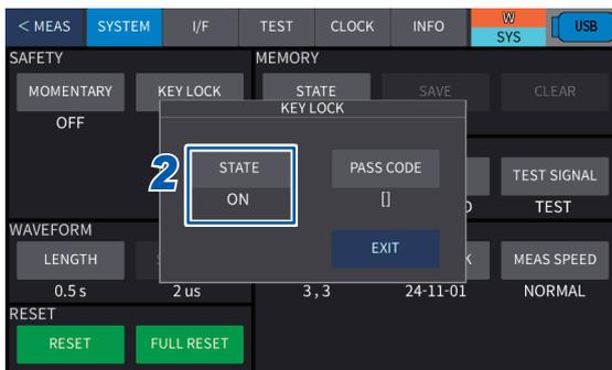
**2** Switch between **[ON]** and **[OFF]** under **[STATE]**.
