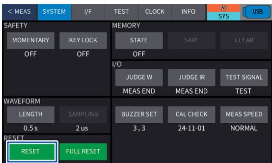
**1** Press **[SYSTEM]** > **[RESET]** on the measurement screen.
