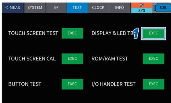
**1** Press **[SYS]** > **[TEST]** > **[EXEC]** of **[DISPLAY & LED TEST]** on the measurement screen.
