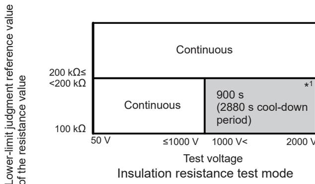
The cool-down time shown in parentheses is required after the maximum voltage output time.
