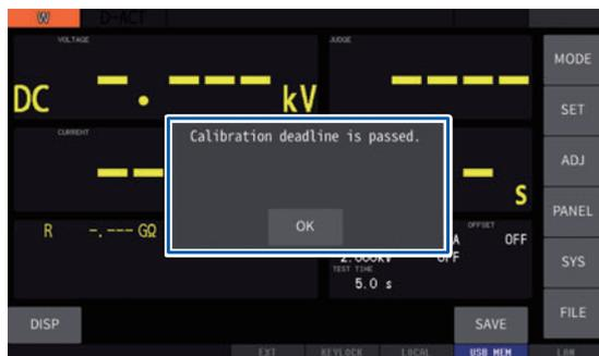
A warning message is displayed when the instrument is turned on after the calibration expiration date.
