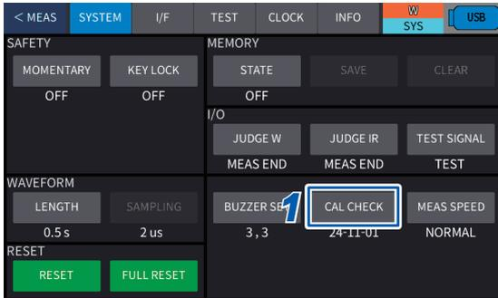
**1** Press **[SYS]** > **[SYSTEM]** > **[CAL CHECK]** on the measurement screen.
