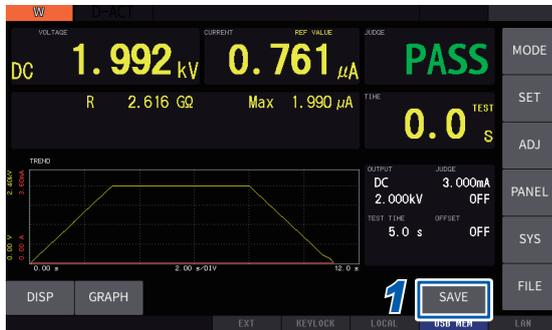
**1** After finishing a measurement, press **[SAVE]** on the measurement screen.
