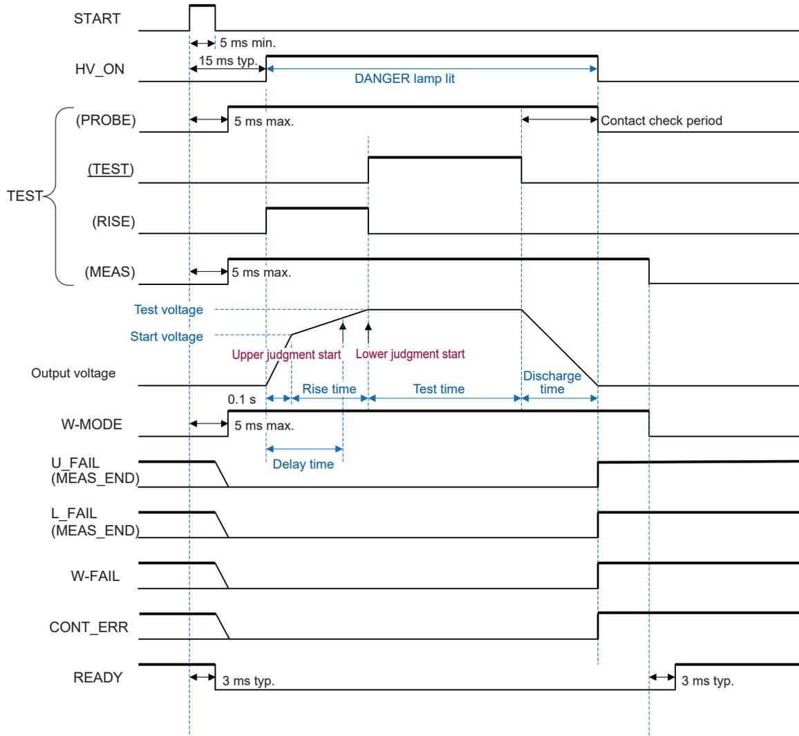
**IR test (fail judgment): With delay time setting (delay time < rinse time), without contact check, insulation resistance test end mode time**
