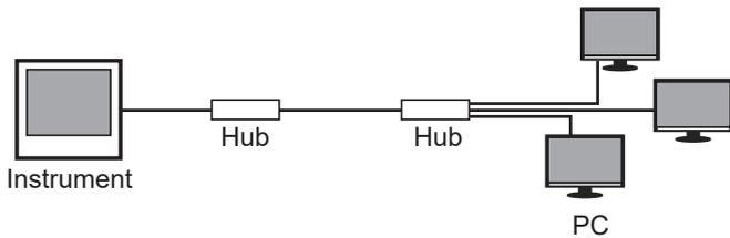
**Connecting multiple instruments to a single PC**
