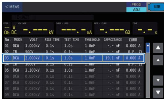
When measurement begins, only the test of the specified step is performed.
