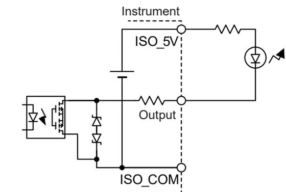
**Connection to programmable controller (negative common inputs)**
