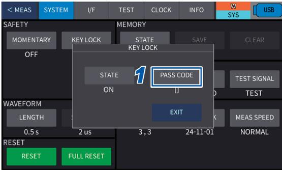
**1** When the key lock state setting is on, press **[PASS CODE]**.
