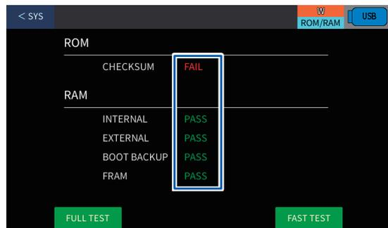
When the test has finished, the test results are displayed.
