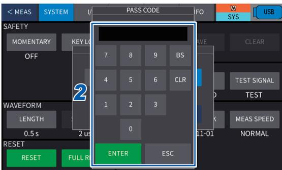
**2** Enter the pass code using the numeric keypad and then press **[ENTER]**.
