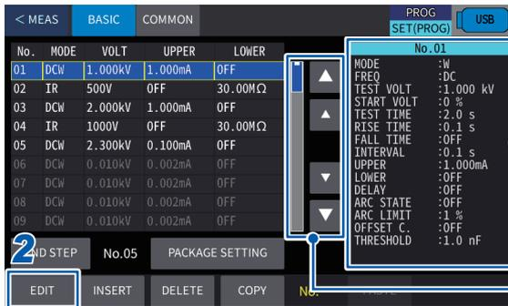
Displays the test conditions of each step.
