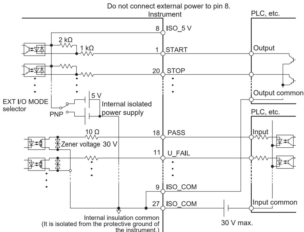
The instrument uses ISO\_COM for the common terminal for both the input and output signals.
