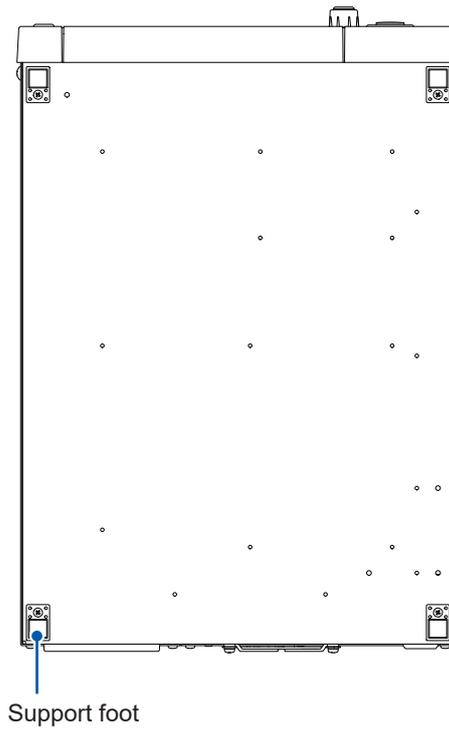
Leave at least 50 mm of space between the installation surface and the instrument vents. (p. 17)
