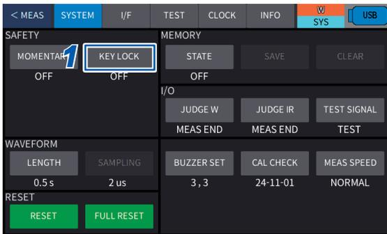
**1** Press **[SYSTEM]** > **[KEY LOCK]** on the system screen.
