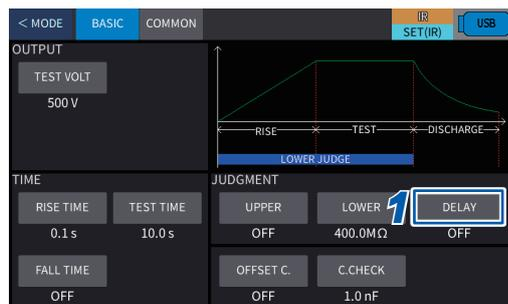
1 Press [BASIC] > [DELAY] on the setting screen.
