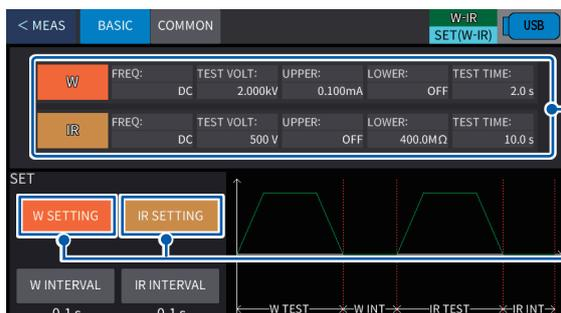
The current test conditions set in the withstand voltage test mode and insulation resistance test mode are displayed.
