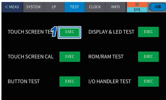
**1** Press [**SYS**] > [**TEST**] > [**EXEC**] of [**TOUCH SCREEN TEST**] on the measurement screen.
