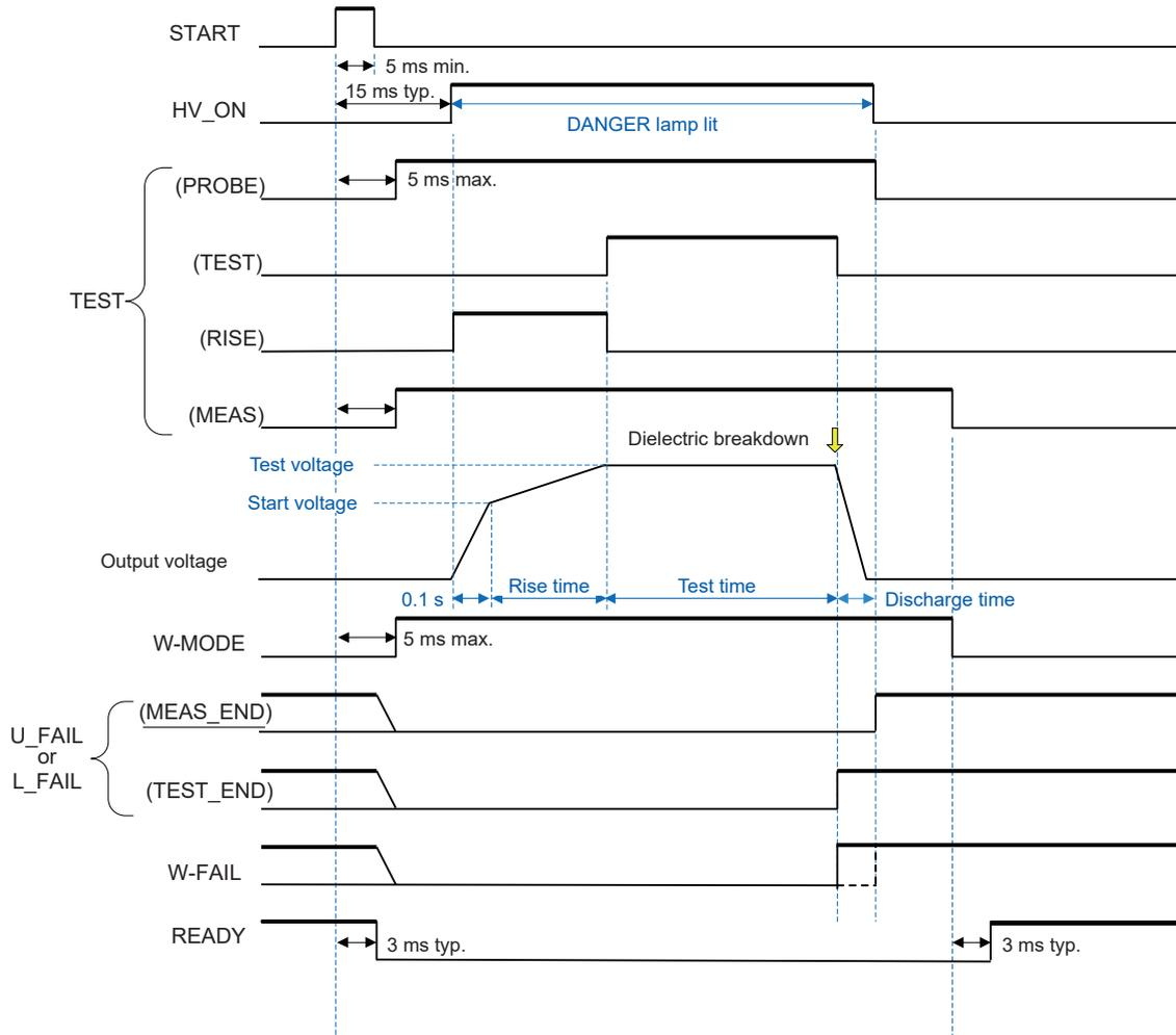
**DCW test (fail judgment): With delay time setting (delay time < rinse time) and contact check (contact error)**
