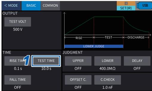
**1** Press **[BASIC]** > **[TEST TIME]** on the setting screen.
