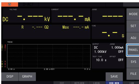
**1** Press **[PANEL]** on the measurement screen.
