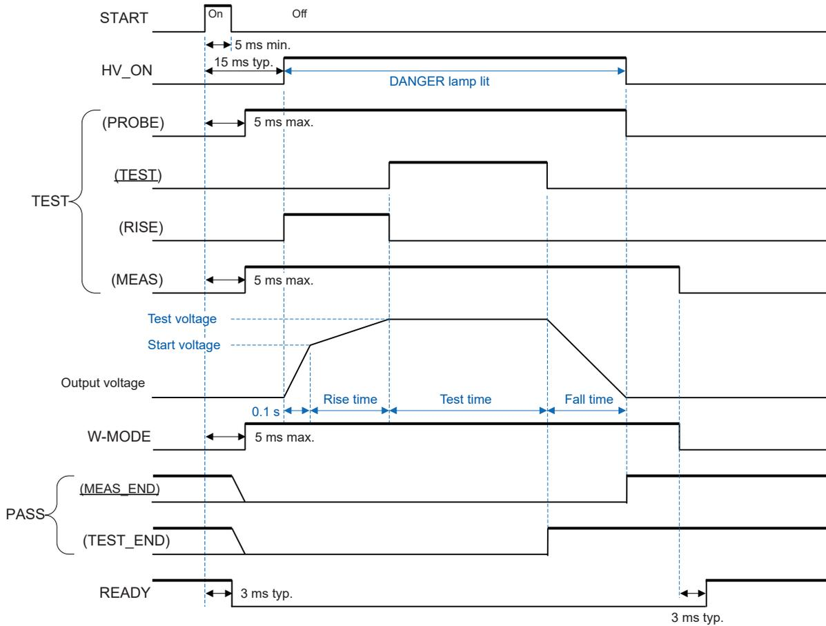
**IR test (pass judgment): With contact check (good contact)**
