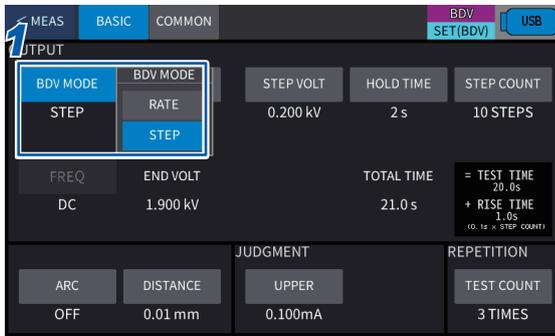
**1** On the setting screen, press **[BASIC]** > **[BDV MODE]** to set the test method to **[RATE]**.
