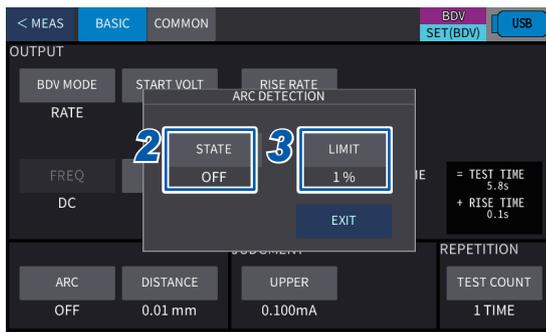
**2** Switch **[ON]** between **[OFF]** under **[STATE]**.
