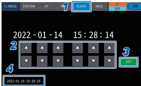
**1** Press **[SYS]** > **[CLOCK]** on the measurement screen.
