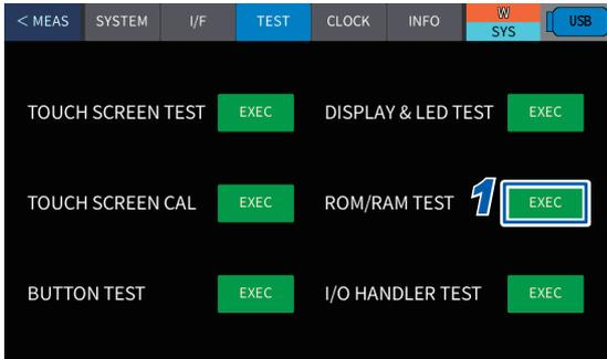
**1** Press [SYS] > [TEST] > [EXEC] of [ROM/RAM TEST] on the measurement screen.
