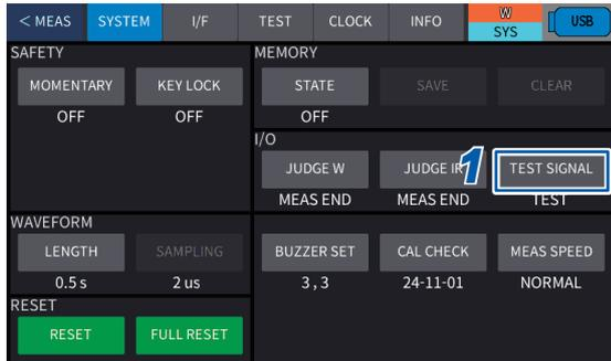
**1** Press [SYSTEM] > [TEST SIGNAL] on the system screen.
