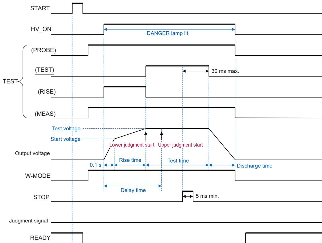
IR test (forced termination with the **STOP** button): With delay time setting (delay time < rinse time)
