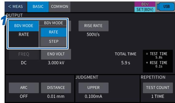
1 Press **[BASIC]** > **[BDV MODE]** to set the test method to **[STEP]**.
