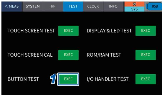
**1** Press **[SYS]** > **[TEST]** > **[EXEC]** of **[BUTTON TEST]** on the measurement screen.
