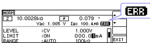
If the voltage or current which is applied to the sample under test exceeds the limit value (the current exceeding the limit value flows through the sample even when the open-circuit voltage is set to minimum value.)
