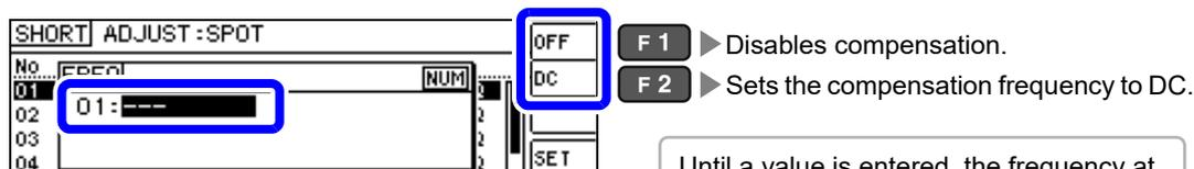
Until a value is entered, the frequency at which spot compensation was previously performed is displayed.
