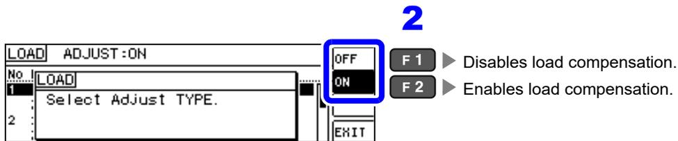
**5** Press the **EXIT** key to enable the load compensation setting and return to the Edit screen.
