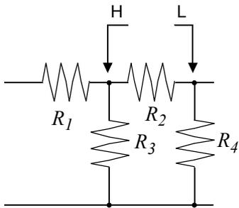
Referring to the following figure, when measuring a resistance value for the resistor  $R_2$ , even if the tips of the two probes are contacted against the ends of the resistor  $R_2$ , considering the sum of the current flowing through the resistor  $R_2$  and the current flowing through the resistors  $R_3$  and  $R_4$ , what is obtained is the resistance value for the parallel combination:
