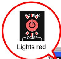
Disconnect the power cord from the outlet to extinguish the POWER button light. When power is turned on again, operation resumes with the same settings as when last turned off.
