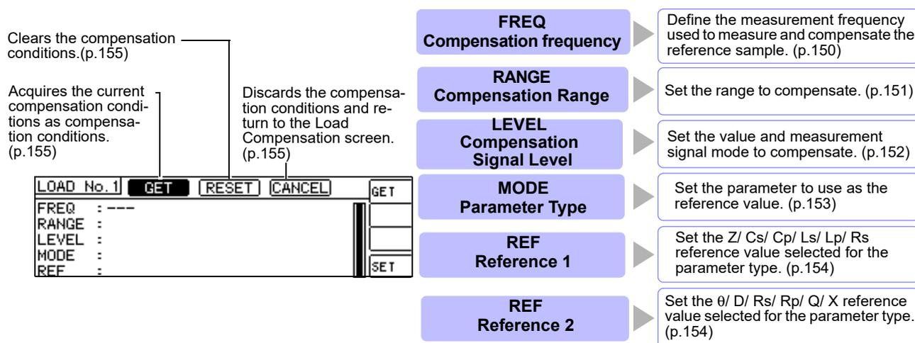
The compensation coefficient is computed from the reference values of Z and  $\theta$  obtained from the set values and the actual data acquired from the reference sample at each of the compensation frequencies.
