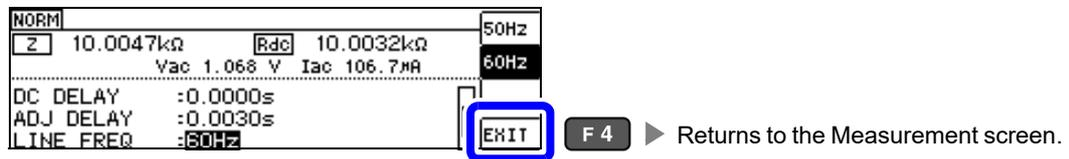
**NOTE** It is necessary to set the line frequency for the power source being used by the instrument in order to reject noise. Set the frequency of the commercial power supply you are using before performing measurements. Failure to set the line frequency correctly will result in unstable measurement values.
