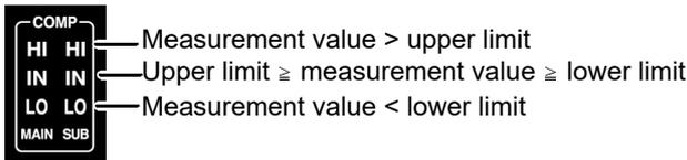
When the comparator measurement results for the main and sub parameters are IN, the IN indicator turns green. When they are HI or LO, the HI or LO indicator turns red.
