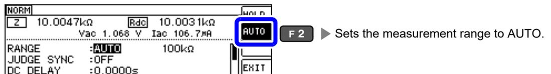
Outside the accuracy guarantee range, AUTO ranging may not function properly, preventing a range from being selected. If this occurs, check the accuracy guarantee range in "10.2 Measurement Range and Accuracy" (p.200) and change the measurement conditions.
