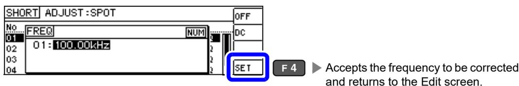
Accepts the frequency to be corrected and returns to the Edit screen.
