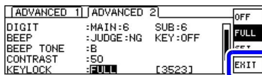
**F 4** ► Enables key lock mode and returns to the Key Lock screen. (p.12)
