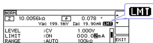
If the test signal level which is being applied to the sample under test exceeds the limit value. Then the test signal level is stopped changing.
