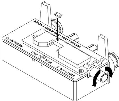
For the connection procedure of the test sample, refer to the instruction manual supplied with the fixture.
