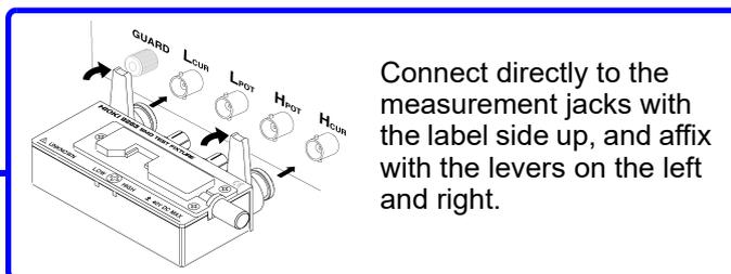
Connect directly to the measurement jacks with the label side up, and affix with the levers on the left and right.
