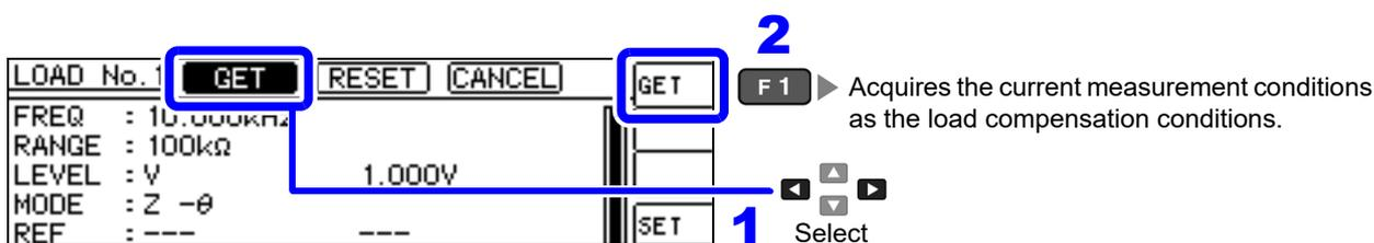
**NOTE** In the above example, loading the measurement conditions with GET causes MODE to be initialized to Z-θ.
