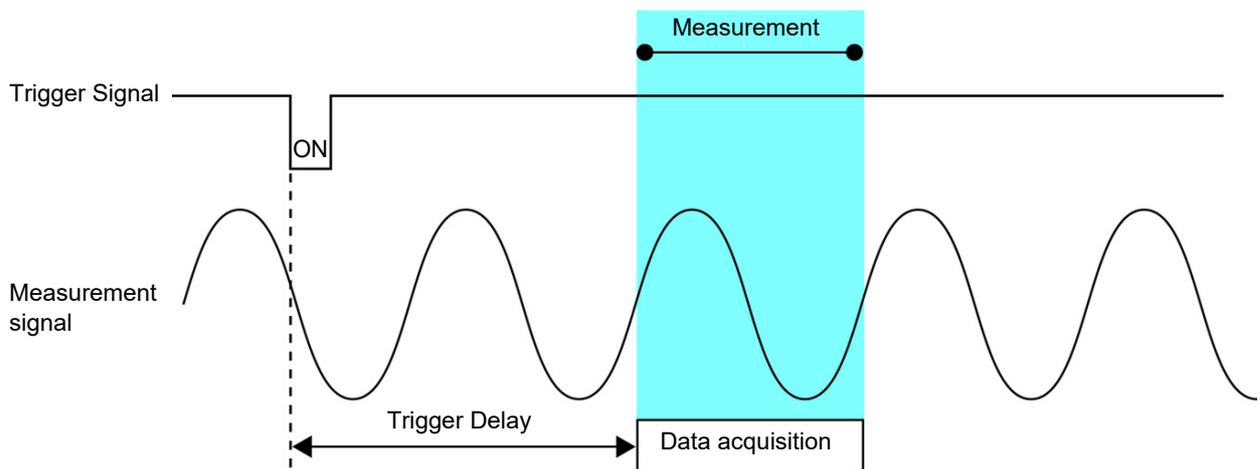
Trigger delay: ON; Trigger synchronous output: ON
