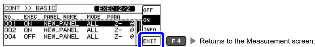
**NOTE** You can select up to two panels. Attempting to select three or more panels will cause the instrument to beep. To change panels, first set the panel you wish to not use to off.
