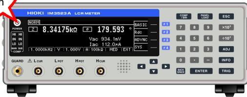
To ensure that measurements fulfill the degree of accuracy described in the specifications, allow the instrument to warm up for at least 60 minutes after it is turned on.
