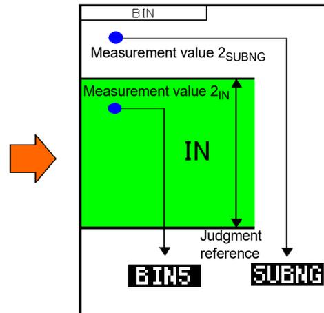
In BIN judgment, a judgment is made based on the main measurement value first, and then the result of a judgment using the sub measurement value is output. In the above example, **OUT** is displayed since main measurement value 1 did not fulfill any of the set judgment standards. Main measurement value 2 was the first to fulfill the standard, and **SUBNG** is displayed since the judgment standard set for BIN5 was fulfilled.
