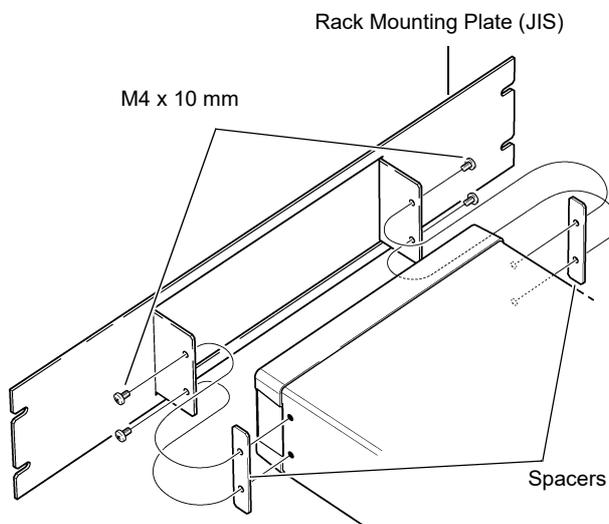
**When installing into the rack, reinforce the installation with a commercially available support stand.**
