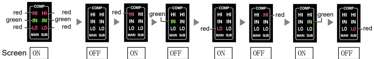
If the entire screen is not the same color or an LED fails to light up, the instrument needs to be repaired. Contact your dealer or Hioki representative.
