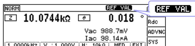
If the measurement value is outside the accuracy guarantee, **[REF VAL]** will be displayed at the top of the screen. Check the accuracy guarantee range in "10.2 Measurement Range and Accuracy" (p.200) and either change the measurement conditions or make the measurement value a reference value.
