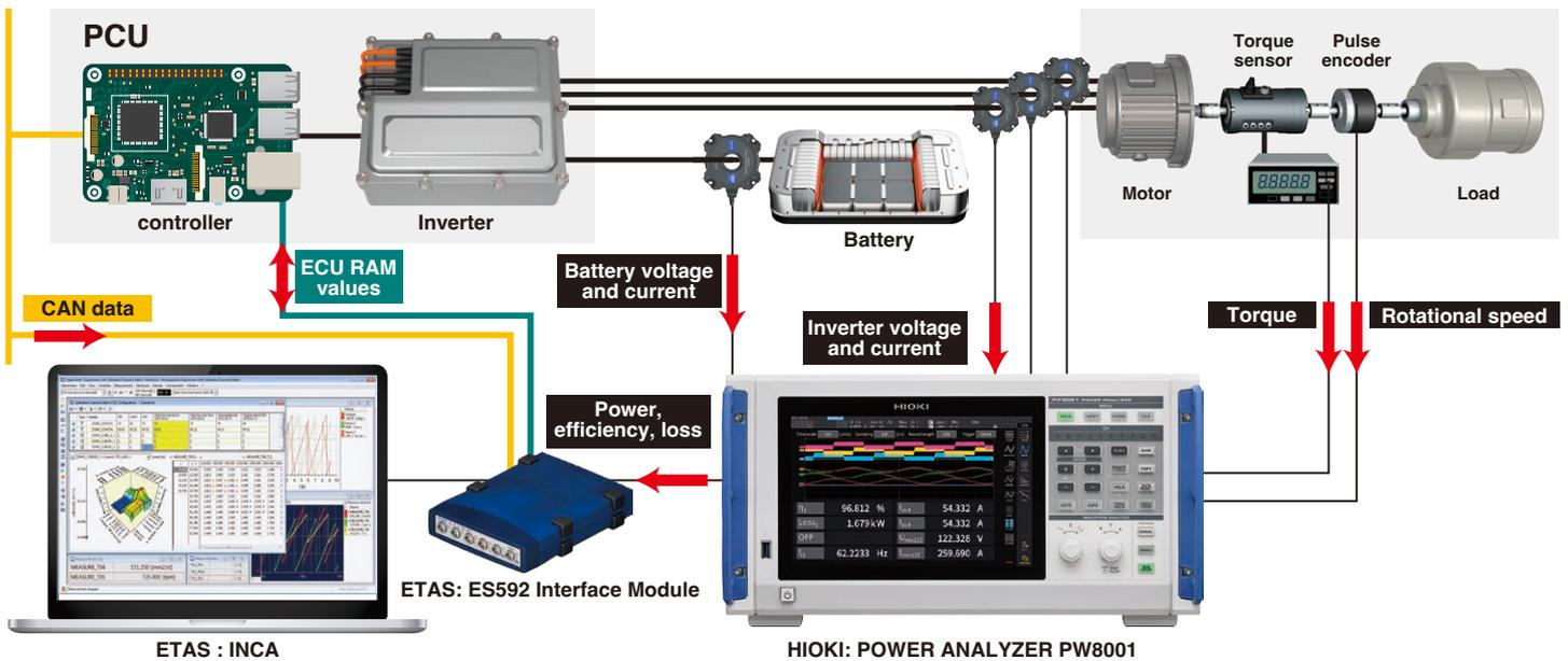
Fast PCU calibration with accurate power measurements
