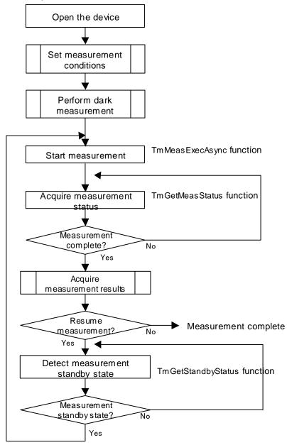
The following diagram illustrates the timing of instrument and library function operation. For more detailed information about instrument operation timing, see "4.2 Timing Chart" in the TM6101 LED Optical Meter Instruction Manual.
