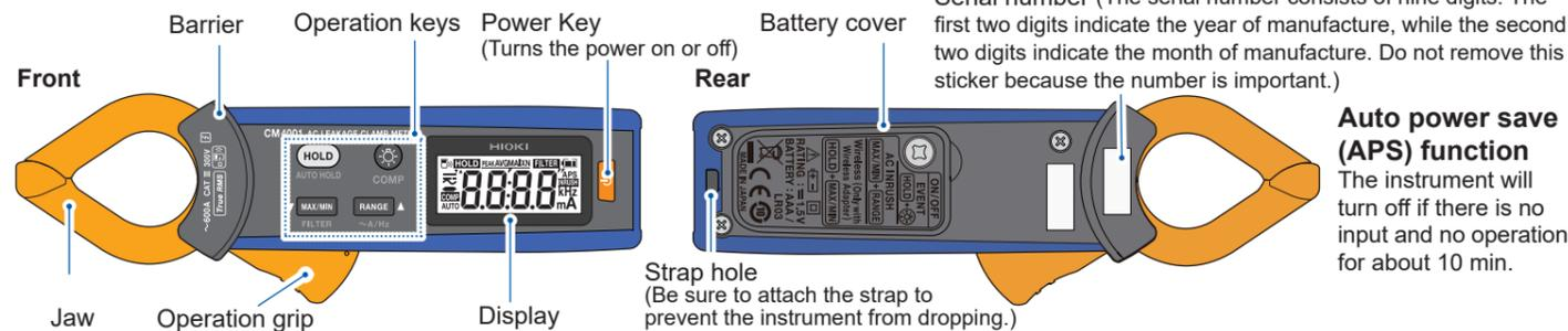
Serial number (The serial number consists of nine digits. The first two digits indicate the year of manufacture, while the second two digits indicate the month of manufacture. Do not remove this sticker because the number is important.)
