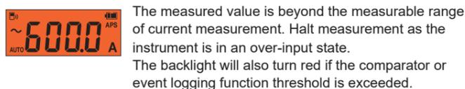
The measured value is beyond the measurable range of current measurement. Halt measurement as the instrument is in an over-input state. The backlight will also turn red if the comparator or event logging function threshold is exceeded.
