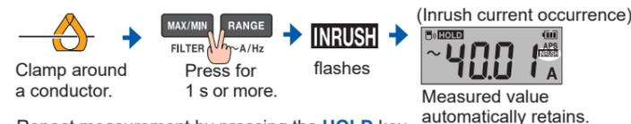
Repeat measurement by pressing the **HOLD** key. Revert to normal measurement by pressing and holding the **MAX/MIN** key and **RANGE** key simultaneously for 1 s or more. The inrush range is fixed at the range during current measurement. Specifically, the inrush range is fixed to the 600.0 A range when using the auto range for current measurement and to the 600.0 mA range when using the 60 mA range for current measurement.
