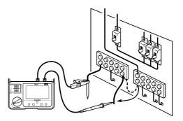
Ex. Checking the continuity of ground wiring
