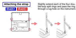
Pass the ring on both ends of the supplied strap through each of the four holes in the instrument.
