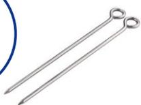
Since variations in the thickness of auxiliary earthing rods cause almost no change in their grounding resistance, the FT6031-50 uses thinner rods that are easier to drive into the ground.
