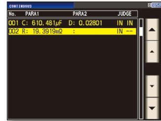
C-D (120 Hz) and low ESR (100 kHz) measurement can be performed for functional polymer capacitors.
