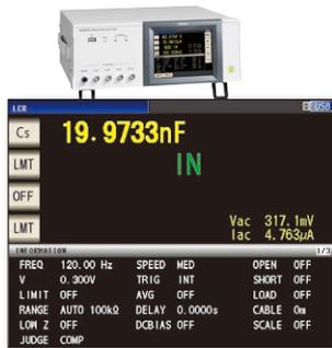
LCR mode Cs display screen (1 kHz measurement)
