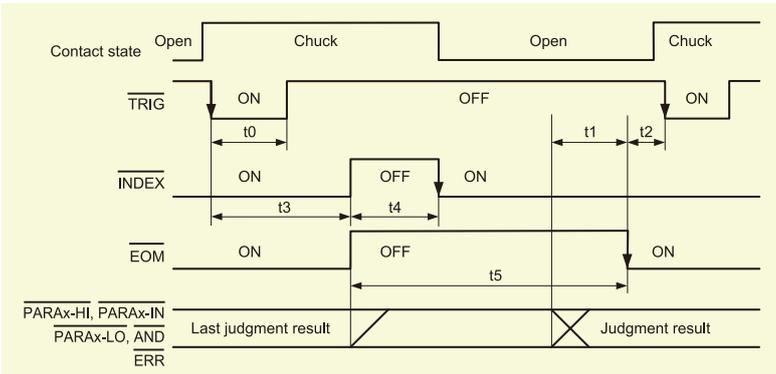
t0: Minimum time for trigger signal: 0.3 ms or longer \*1
