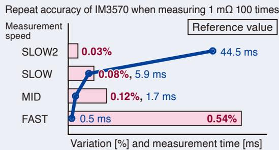
A one-digit improvement in repeat accuracy during low-impedance measurement has been achieved compared with previous Hioki products. For example, when the condition is 1 mΩ (1 V, 100 kHz) and the measurement speed is MED, stable measurement with a repeat accuracy (variation)\* of 0.12% is possible, making this instrument suitable for 100 kHz ESR measurement.
