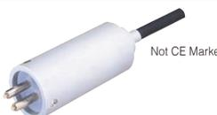
Electrode for surface resistance of curved samples such as resin and rubber processed goods, TV cathode tubes or small samples. Surface resistance can be measured by pressing the rubber tips at the tip onto the sample. Measure electrodes up to 10<sup>11</sup> Ω at 10 mm (0.39 in) intervals or greater.
