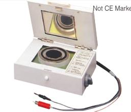
Sample of 100 mm (3.94 in) square by up to 8 mm (0.31 in) in thickness is measurable. The main electrode dia. is 50 mm (1.97 in) and inner & outer dia. of ring electrode are 70 mm (2.76 in) & 80 mm (3.15 in) respectively. Measurement voltage becomes "OFF" while the lid is open to ensure safety. A selector switch allows selection of voltage or surface resistivity.
