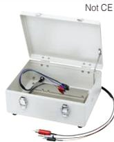
This is used as a sample accommodation box during measurement of a high-insulation resistance samples, or inductive or capacitive samples to perform electromagnetic shielding. When used in combination with mass electrode SME-8320, the electrode can be used as a counter electrode or a guard electrode. When measuring electronic components such as capacitors and transducers, external noise and leakage currents are prevented to ensure stable measurement.
