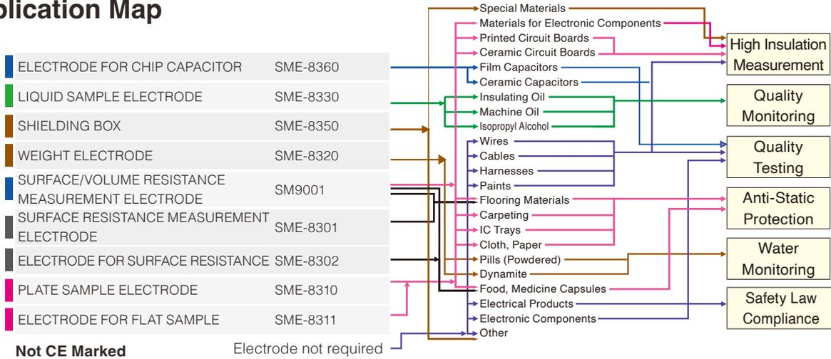
\*When connecting electrodes and shield boxes to SM7110/SM7120, note that CONVERSION ADAPTER (Custom order product Z5010) or a change of connectors is required. Please contact your local Hioki distributor for assistance.
