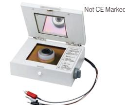
Sample of 40 to 100 mm (1.57 to 3.94 in) square by up to 8 mm (0.31 in) in thickness is measurable. The main electrode dia. is 19.6 mm (0.77 in) and inner & outer dia. of ring electrode are 24.1 mm (0.95 in) & 28.8 mm (1.13 in) respectively. Measurement voltage becomes "OFF" while the lid is open to ensure safety.
