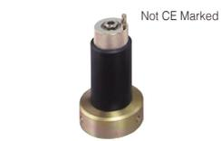
Electrode for liquid samples which is electrically guarded. Total volume is 25ml. Capacitance between main and counter electrode is approx. 45 pF. Electrode constant is approx. 500 cm (16.41 ft). Distance between both electrodes is 1 mm (0.04 in). Outer dia. is 36 mm (1.42 in), height is approx. 140 mm (5.51 in). Measure resistance up to 10<sup>19</sup> Ω (at 1000 V) when used together with Model SM-8220.
