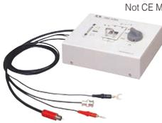
For easily measuring capacitor tip resistance. The jig can be arbitrarily adjusted up to 11 mm (0.43 in) in length (compatible with EIA 0603 [JIS 1608] size or larger), capable of measuring various tip capacitors. When connected to the megohmmeters by an interlock cable, measurement voltage becomes "OFF" while the lid is open to ensure safety. \*The interlock cable must be modified in order to use the product with the SM-8220 series.
