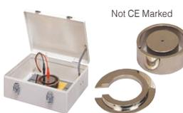
This is an electrode for plate sample for use together with SME-8350 shield box. This electrode enables extremely easy measurement of surface resistivity and volume of sample with coarse surface such as carpets, etc. The main electrode dia. is 50mm (1.97 in), and the ring electrode inner-dia. and outer-dia. are 70mm (2.76 in) and 80mm (3.15 in) respectively.
