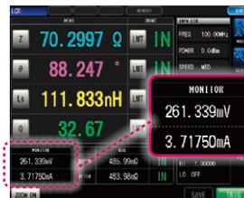
Display the measurement signal level being applied to components in real time.
