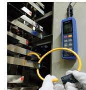
These sensors can be easily routed through confined locations and between cables. The tapered tip is designed so that it can be fed readily through tangled wires. In addition, a magnetic strap\* frees both hands for other tasks.
