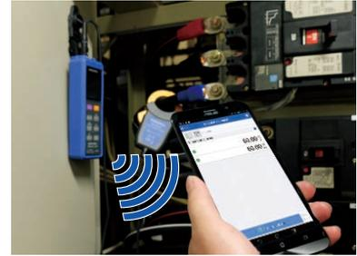
Measurement results will be sent to the tablet wirelessly and displayed.
