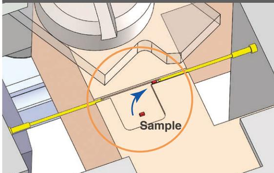
3. Move the control lever to the "CLOSE" position to lock the sample in place.
