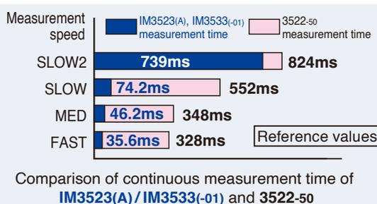
With continuous measurement under varying measurement conditions such as C-D + ESR measurement of capacitors, the total measurement time has been shortened significantly from the previous HIOKI model 3522-50. In addition to the reduction of the time required for individual measurements, the time required to change ranges such as a frequency range has been reduced significantly.
