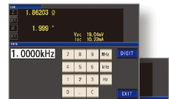
Frequency setting (numeric keypad input and up/down input)
