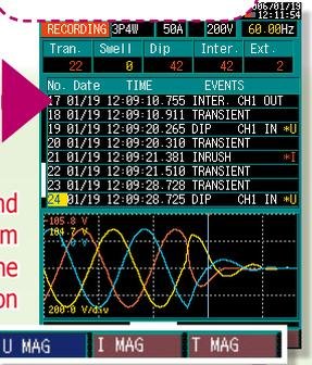
Inrush current fluctuations are captured in RMS at a fast 10ms sampling rate and displayed across a 30-second window
