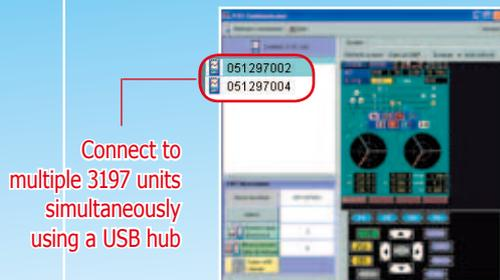
Connect to multiple 3197 units simultaneously using a USB hub
