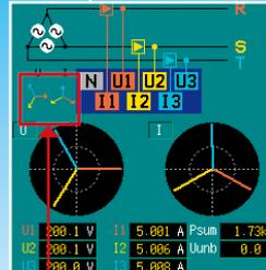
Use the wiring map, vector map and data monitor to check for proper wiring before taking measurements – don't miss out on important power data just because of minor wiring mistakes!
