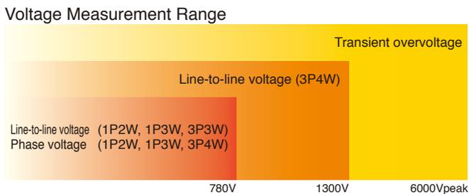
Both low and high voltages can be measured in a single range.
