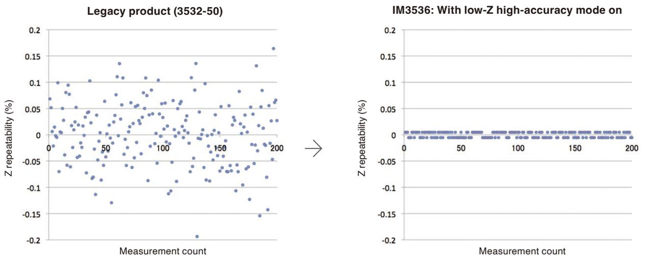
Graphs illustrate the results of measuring a resistance of 1 mΩ 200 times under the following conditions:
