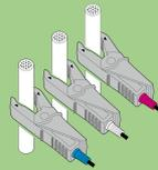
Proper electrical testing requires that all three phases be clamped.
