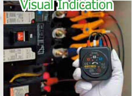
Based on the electrostatic induction theory, the 3129 series Phase Detectors can safely and accurately detect phase sequence in three-phase circuits. Correct sequence is indicated by a crystal clear beeping tune, while bright red LEDs show sequence direction.
