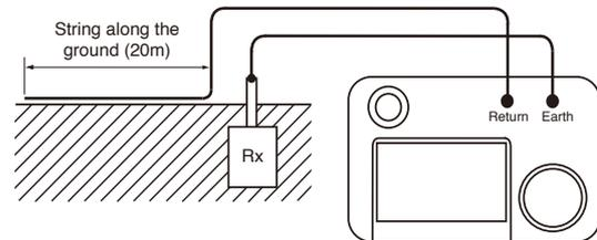
The 3143 is most appropriate for measuring the ground resistance of an individually grounded rod-shaped electrode.
