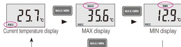
The 3441 and 3442 support temperature management by recording maximum and minimum temperatures in memory. By pressing the MAX/MIN key, you can switch to display of the current maximum and minimum temperatures at any time.
