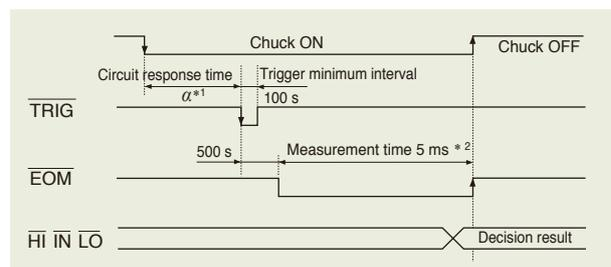
\*1  $\alpha$  depends on the sample and trigger delay.
