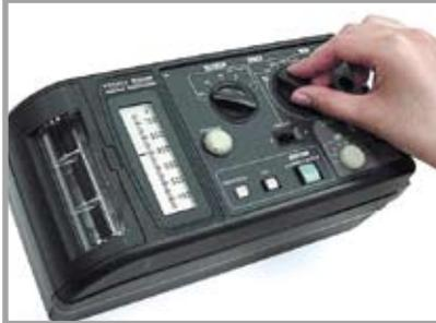
Intuitive analog dials are used to set the input range and paper feed speed. This makes the recorders as easy to operate as a multimeter.
