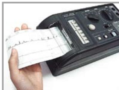
Sensitized recording paper is used, providing clean, quiet recording. Further, HIOKI's RECORDING PAPER 9236-01 and provides superior climate resistance and is much less susceptible to discoloration due to chemical exposure than ordinary thermal recording paper, providing much longer print life.
