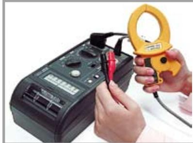
With 2-channel recording, a single instrument can simultaneously record both voltage and current. This is ideal for management and testing of power lines.
