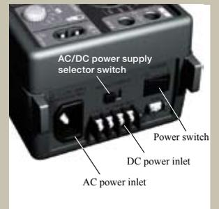
In addition to a universal power AC supply of 100 to 240V, the recorders can operate on 9.5 to 14V DC power supplies. This is useful outdoors and in other field applications.
