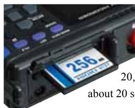
Data is efficiently saved to a CF card. When the HiCORDER is connected to a PC via USB cable, the data is quickly copied from the installed card to the PC: 20,000 waveform screen divisions transfer in about 20 seconds.
