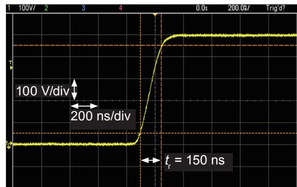
Fig. 3. Example of a rising waveform (500 V).
