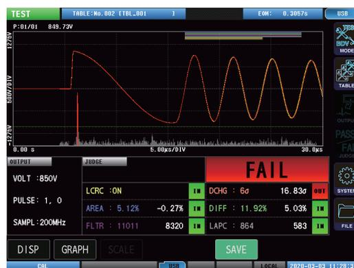
Fig. 7. Waveform graph display screen (with discharge).
