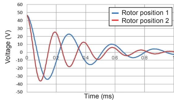
Fig. 12. Voltage waveform variation when rotor is rotated.
