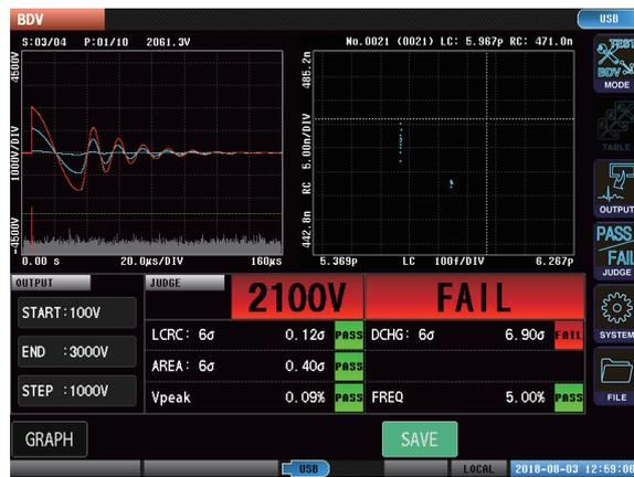
Fig. 9. BDV test screen.
