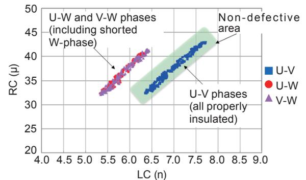
Fig. 13. Distribution of LC and RC values between each phase of a motor whose W-phase is shorted.
