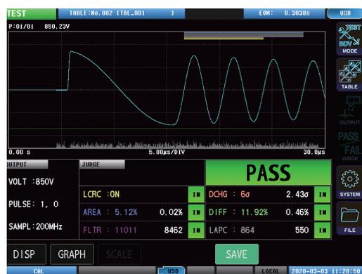
Fig. 8. Waveform graph display screen (without discharge).
