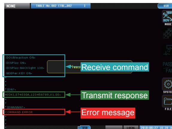
Fig. 11. Communication monitor screen.
