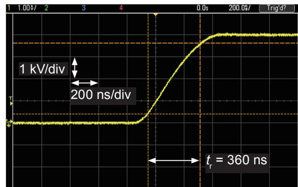
Fig. 4. Example of a rising waveform (4.2 kV).
