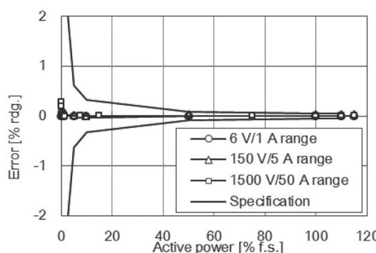
Fig. 8. Active power linearity: AC+DC.
