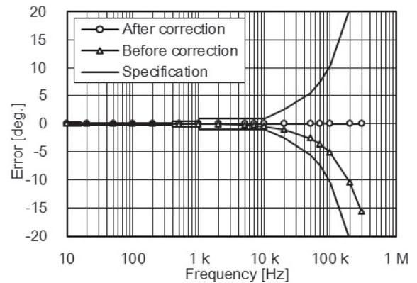
Fig. 2. CT6862 phase characteristics correction.
