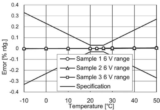
Fig. 13. Voltage temperature characteristics: DC (0% f.s.).
