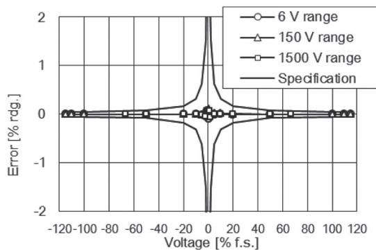
Fig. 3. Voltage linearity: DC.
