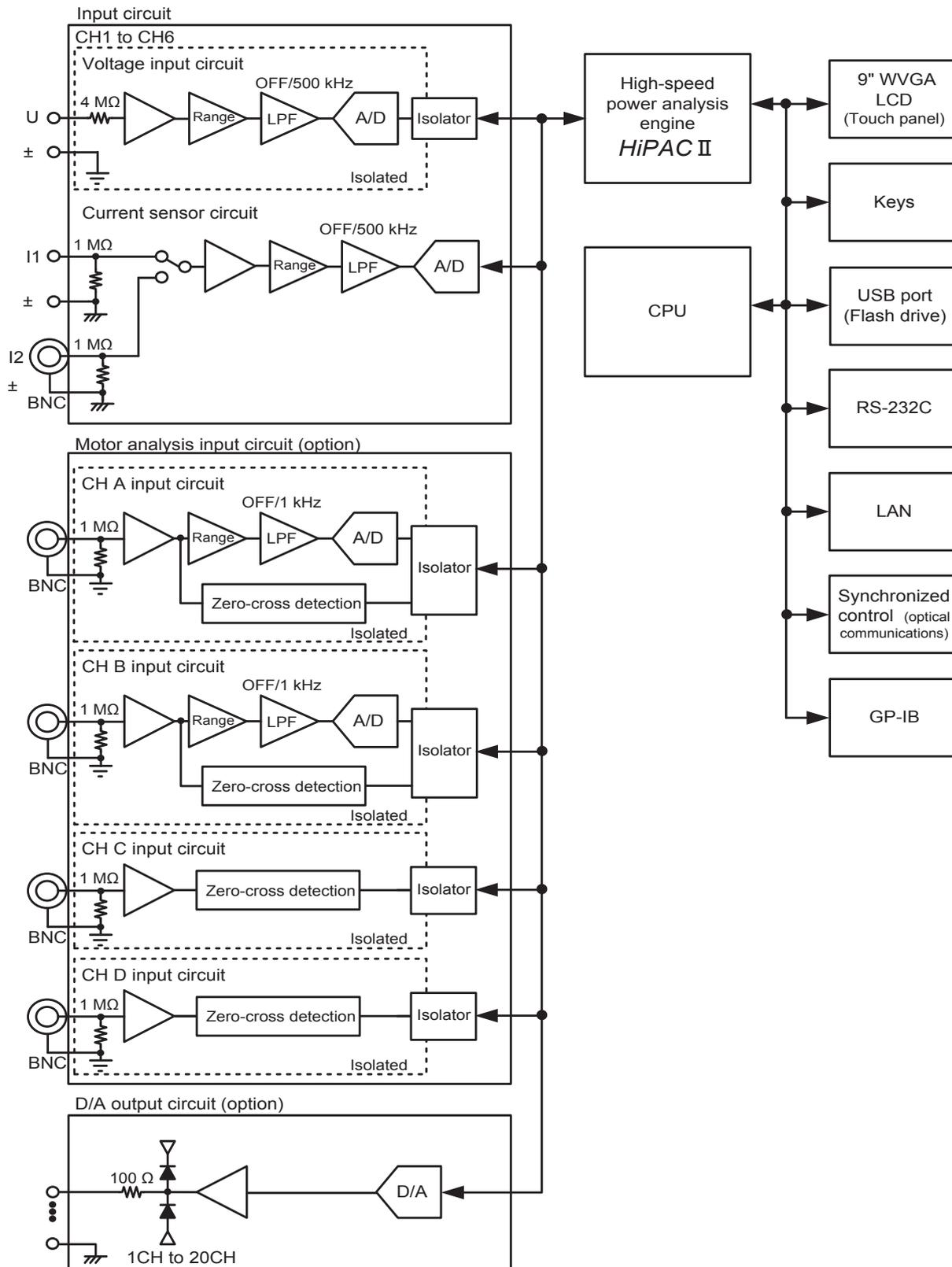
Fig. 1. Block diagram.
