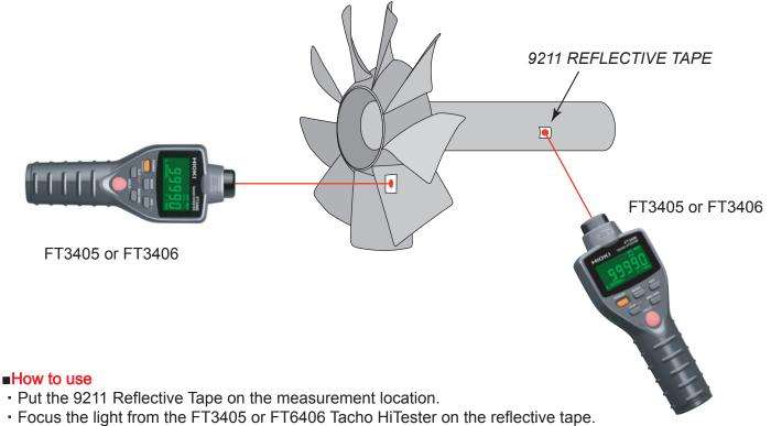
• The measurement distance is 50 to 500 mm and the measurement range is 30 to 99990 rpm.
