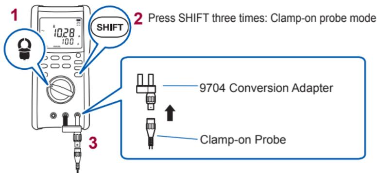
**Set the clamp-on probe and the instrument to the same range.**
