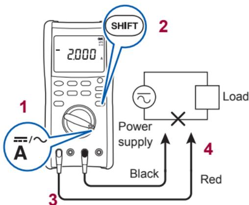
For AC current measurement, the instrument may display zero if the input current is lower than each range's accuracy guarantee range.
