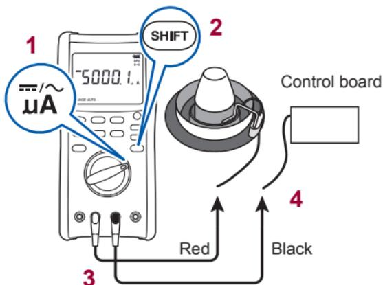
Example: Measuring the current of the burner flame ( $\mu\text{A}$ )
