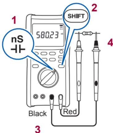
The open terminal voltage is approx. 2.5 V or less. The measurement current (DC) is approx. 96 nA. (p. 93)
