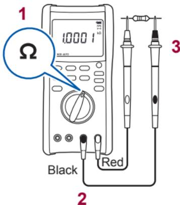
Measurement of inductors, including motors and transformers, may cause unstable auto-range switching. In such a case, set the range manually (p.61). Moreover, if a capacitive component is connected across the object under measurement, its measured value may be incorrect.
