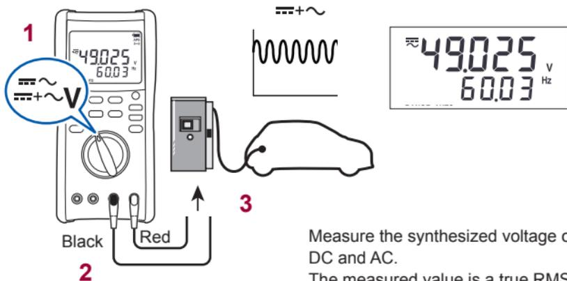
Measure the synthesized voltage of DC and AC.
