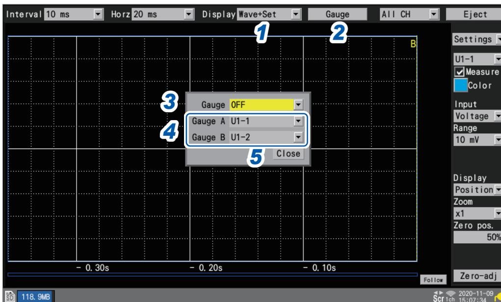
**1** Under **[Display]**, set the display to **[Wave+Set]**, **[Wave]**, or **[Wave+Value]**.
