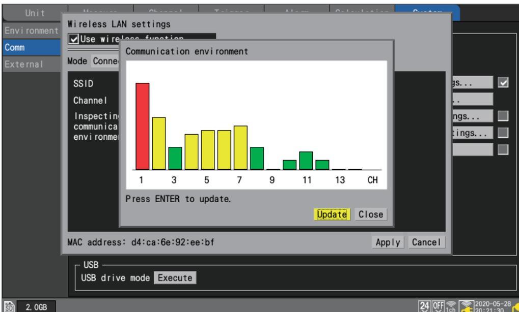
The instrument will indicate the communications congestion level with colors (green, yellow, red). The channel numbers represent [Channel] with the wireless LAN [Mode] setting set to [Wireless unit connection].
