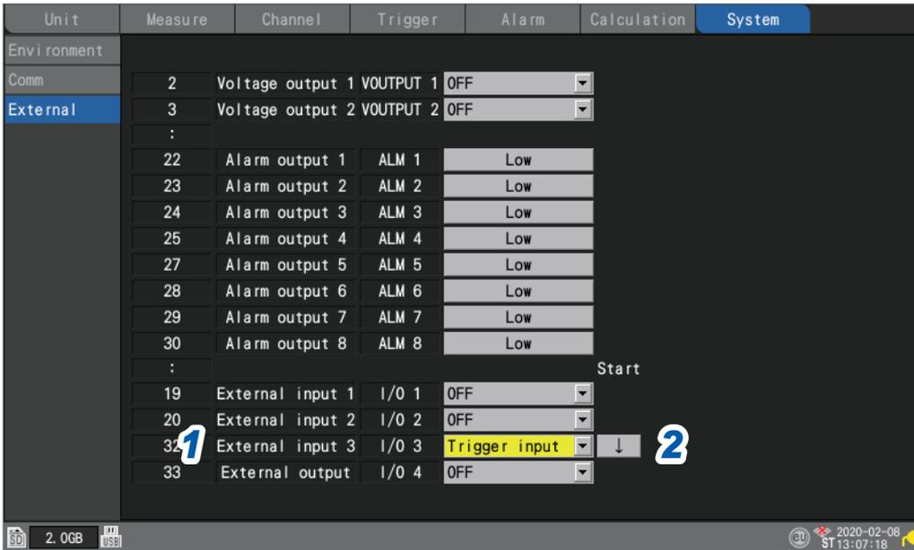
**1** Under **[External input 3]**, set the terminal functionality to **[Trigger input]**.
