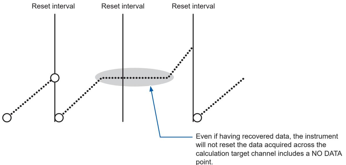
In addition, no reset will be performed when the calculation has already progressed beyond the trigger point upon the recovery. The reset will be performed at the point when the next reset condition is satisfied for the first time since the trigger has activated.
