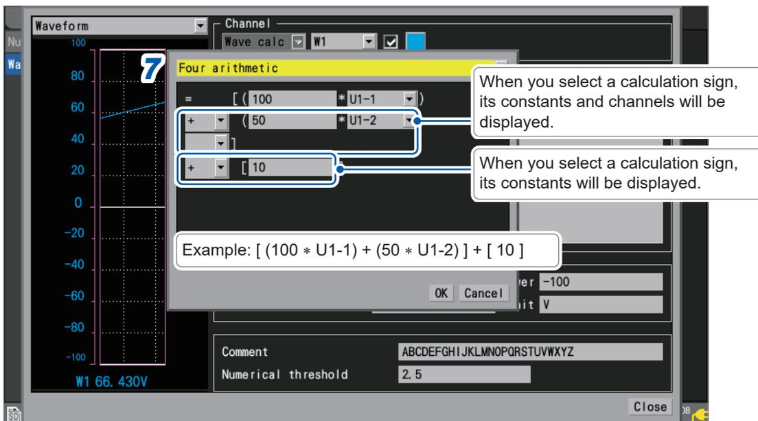
You can select a calculation channel as a target channel; however, you cannot select a calculation channel with a number that is larger than the number of the configured calculation channel.
