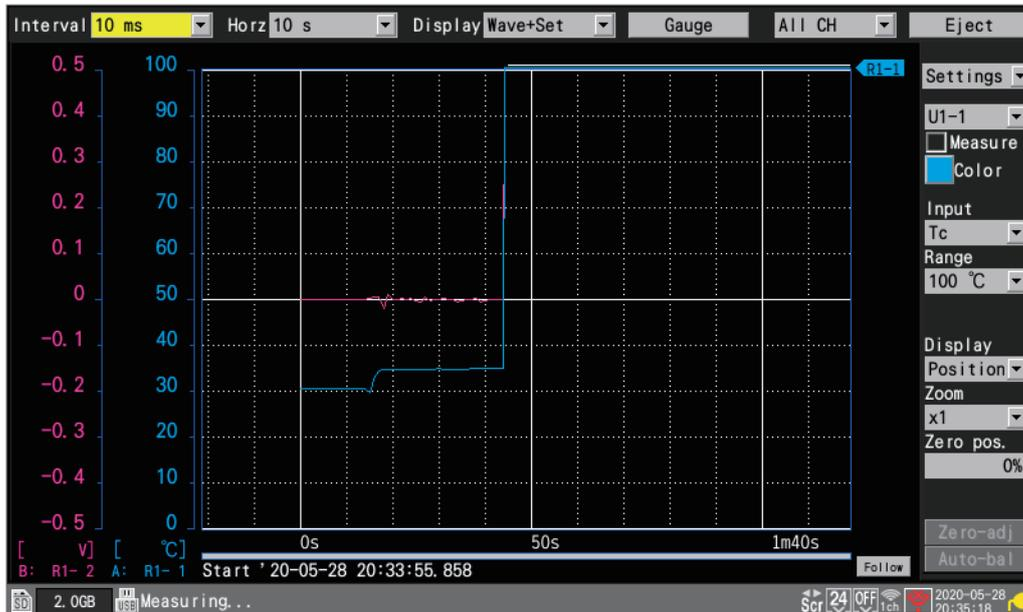
The instrument will halt waveform drawing during disruption of communications between the instrument and the wireless modules and data recovering processes.
