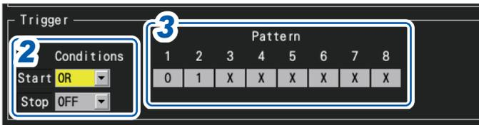
**2** Under **[Conditions]**, select the pattern for activating the trigger.
