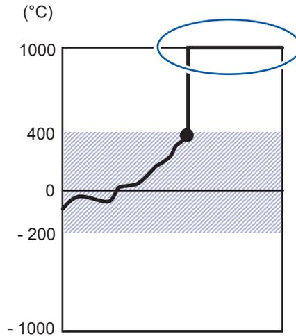
When using wire break detection in thermocouple measurement, values are treated as follows:
