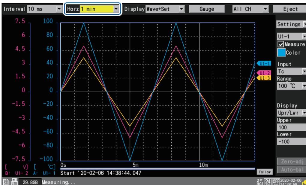
Under **[Horz]**, you can select the time per division. This setting can be changed while measurement is in progress.
