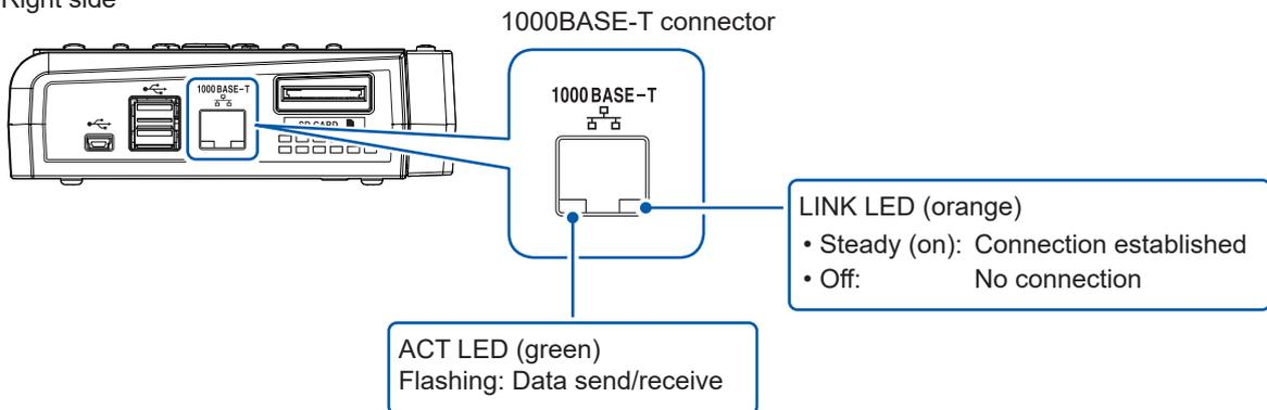
The LINK LED will light up when the instrument has connected to the network, indicating that the connection can be used. If the LED fails to illuminate, there may be a malfunction of the instrument or connected device or a wire break in the LAN cable.
