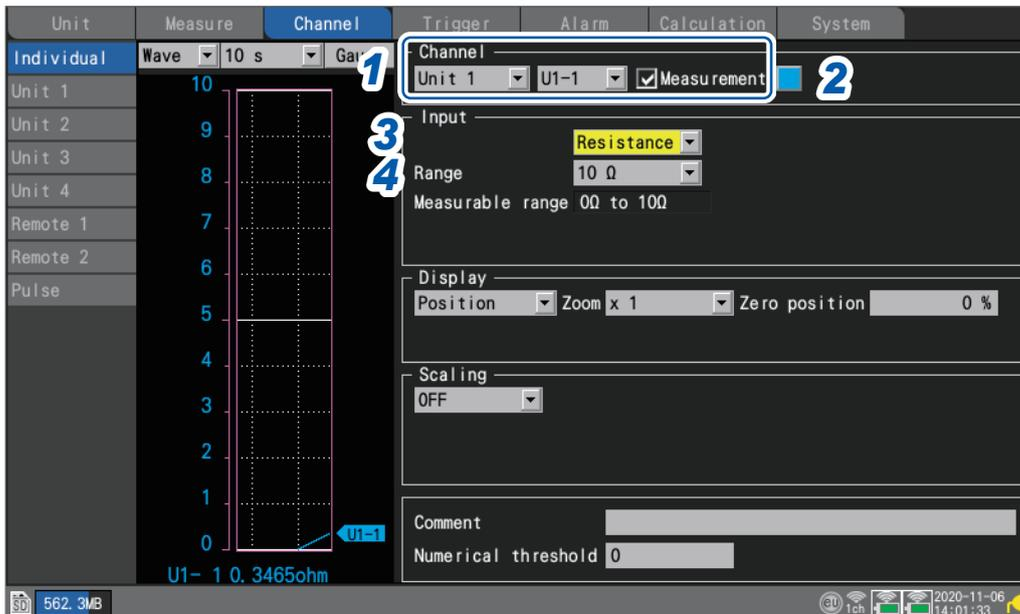
**1** Select the module (Unit) and channel to configure and select the check box. Measurement will not be performed for channels whose check boxes are not selected.
