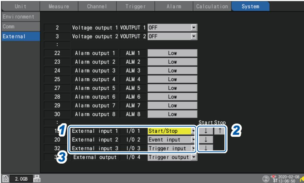
**1** Under **[External input 1]**, **[External input 2]**, and **[External input 3]**, select the terminal functionality.
