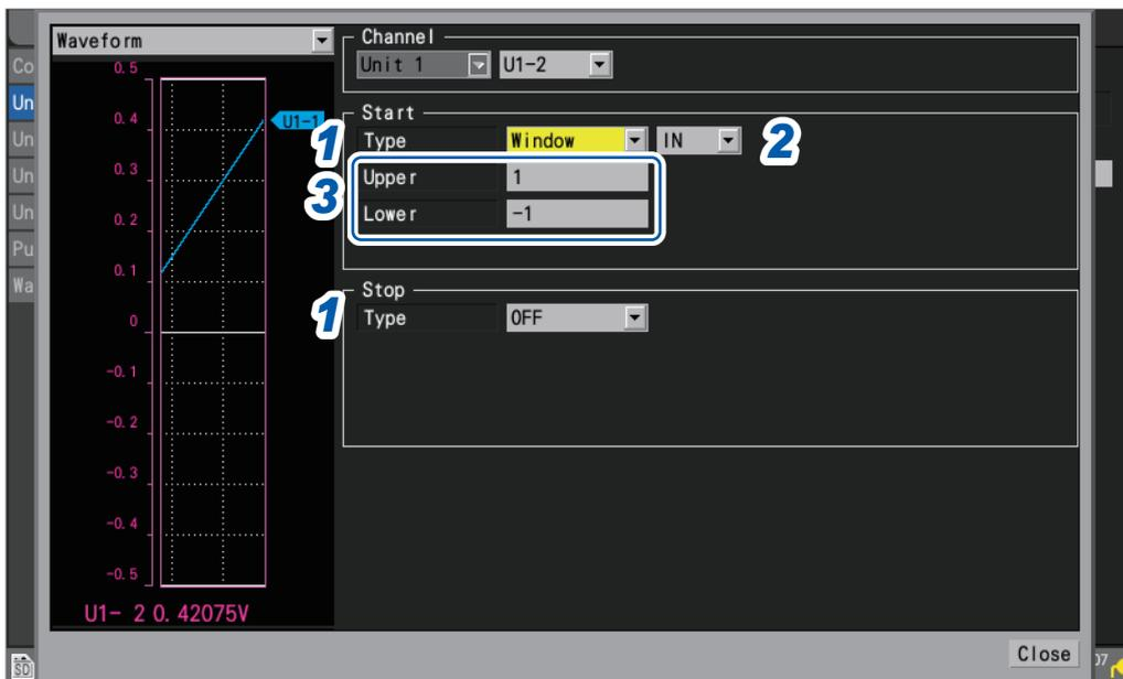
**1** Under [Type] for [Start] or [Stop], set the trigger type to [Window].
