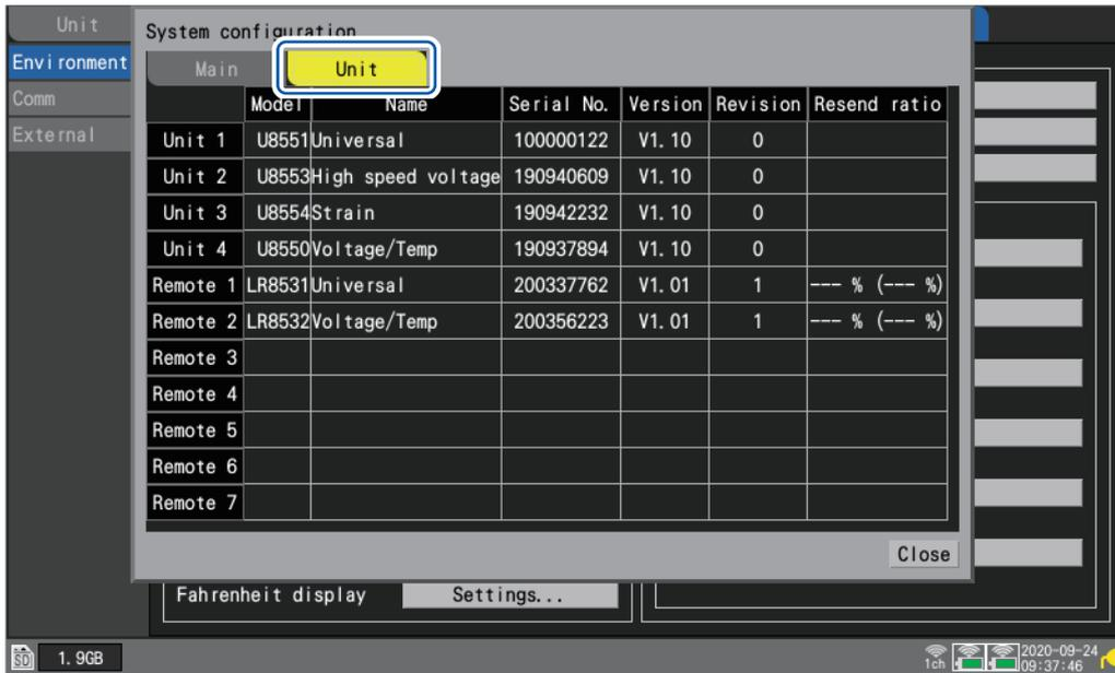
Unit 1 to 4: Plug-in modules; Remote 1 to 7: Wireless modules
