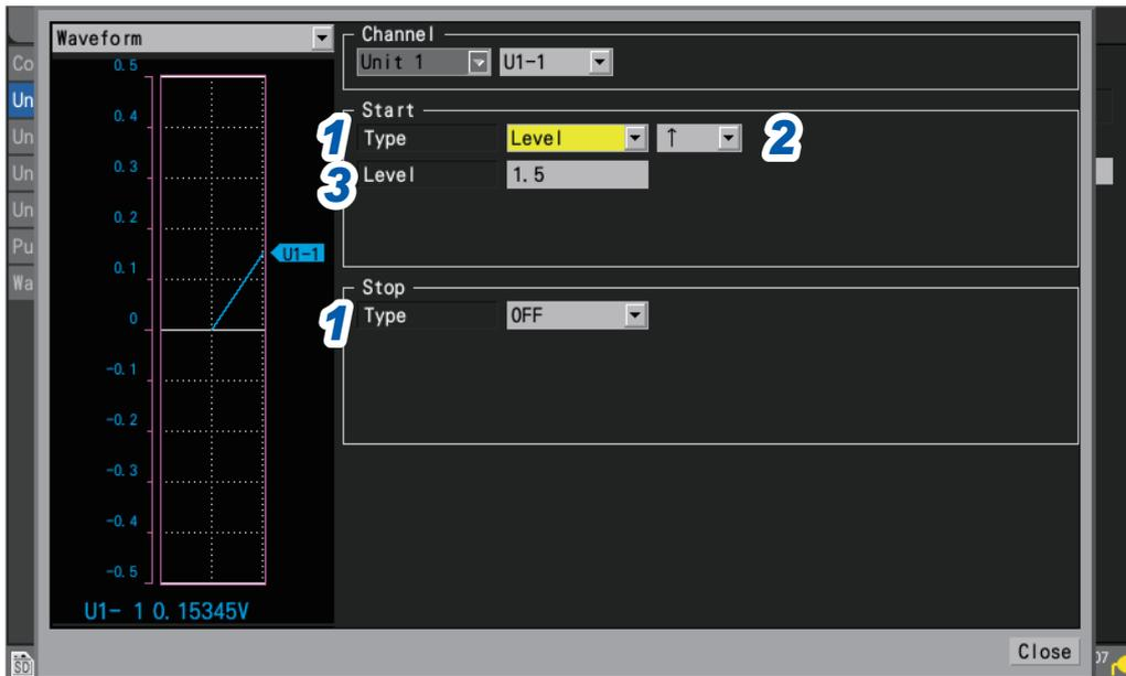
**1** Under [Type] for [Start] or [Stop], set the trigger type to [Level].
