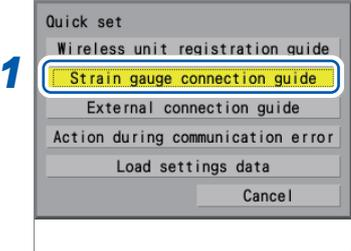
**1** Select [Strain gauge connection guide].
