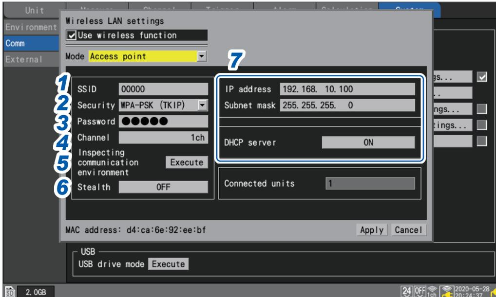
**1** Under [SSID], set an identification name for an access point.
