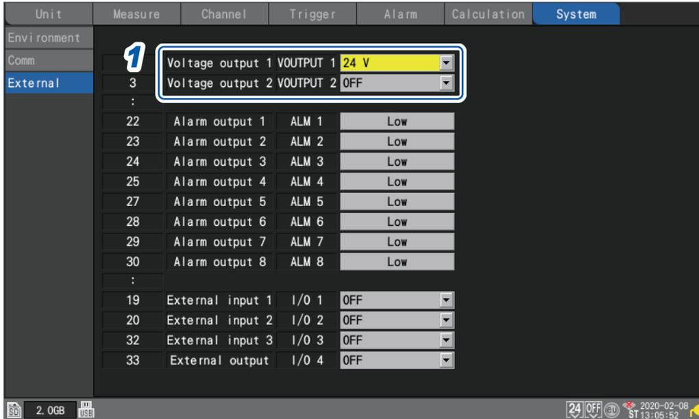
**1** Under **[Voltage output 1]** and **[Voltage output 2]**, select the voltage.
