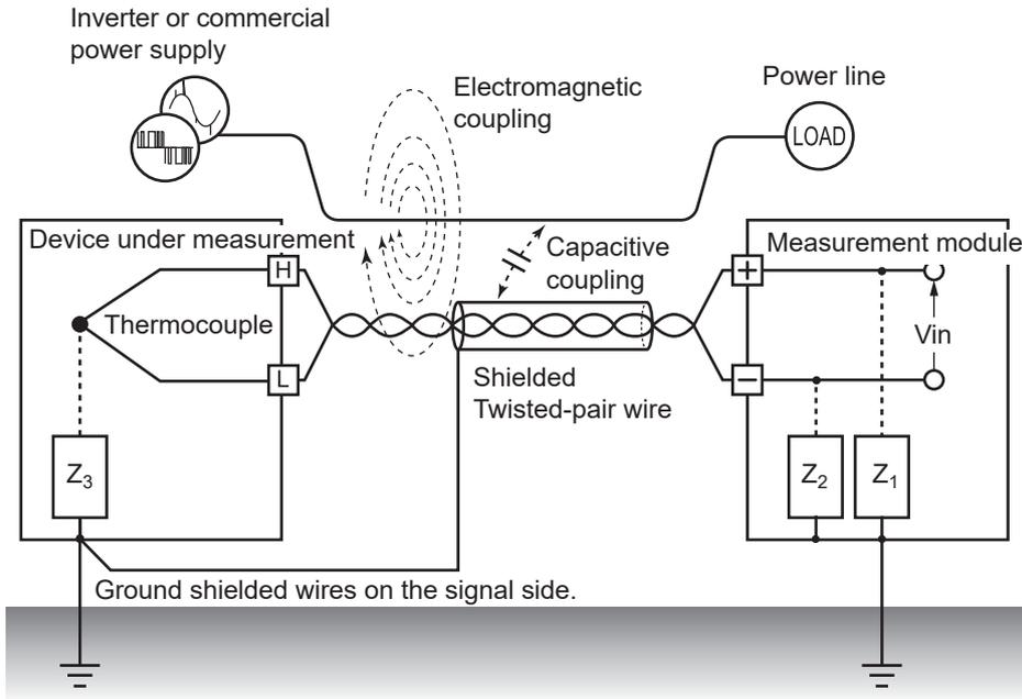
Keep signal lines (thermocouples) away from wires that could serve as sources of noise (power supply lines, etc.). Furthermore, you can block capacitive coupling by shielding and grounding signal lines.
