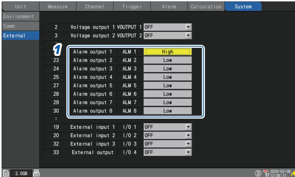
**1** Under **[Alarm output 1]** to **[Alarm output 8]**, select the voltage level you wish to output when outputting an alarm.
