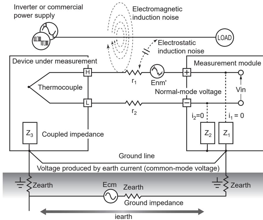
Connect the chassis GND on the signal side to a suitable ground with adequately low grounding resistance.
