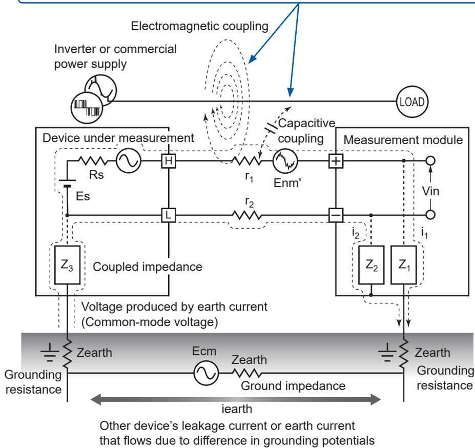
Common-mode noise is caused by ground impedance that is interposed between the ground points of the device under measurement and the measurement module and capacitive coupling between ground lines and noise sources.
