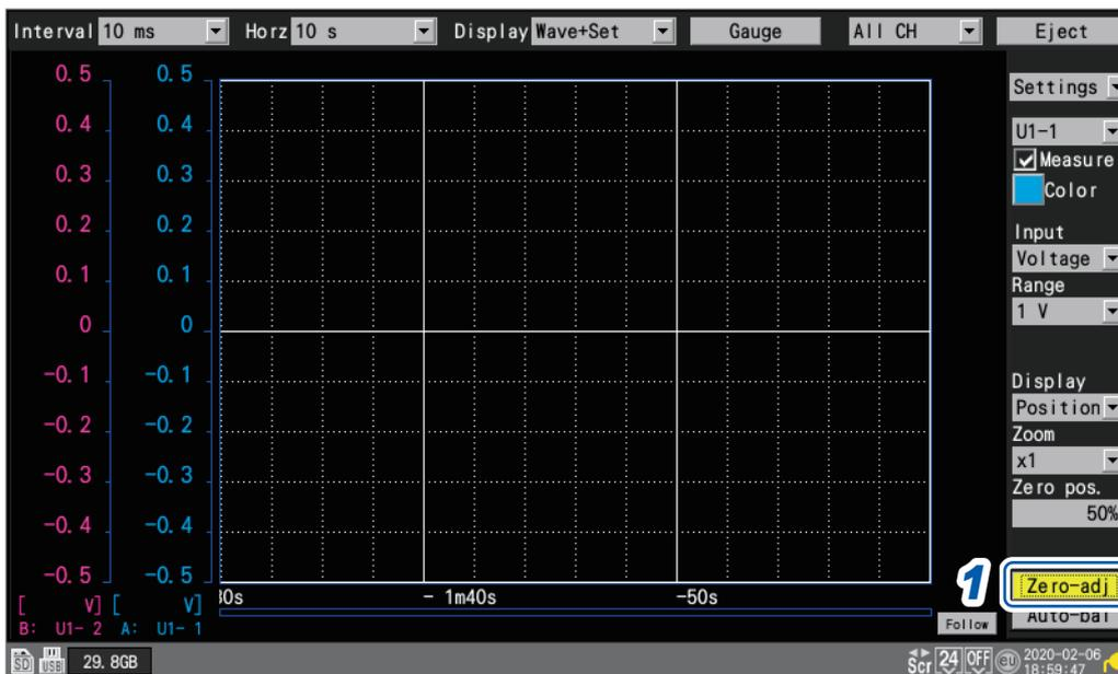
Zero adjustment values are reset when a system reset is performed. Zero adjustment cannot be performed while measurement is in progress.
