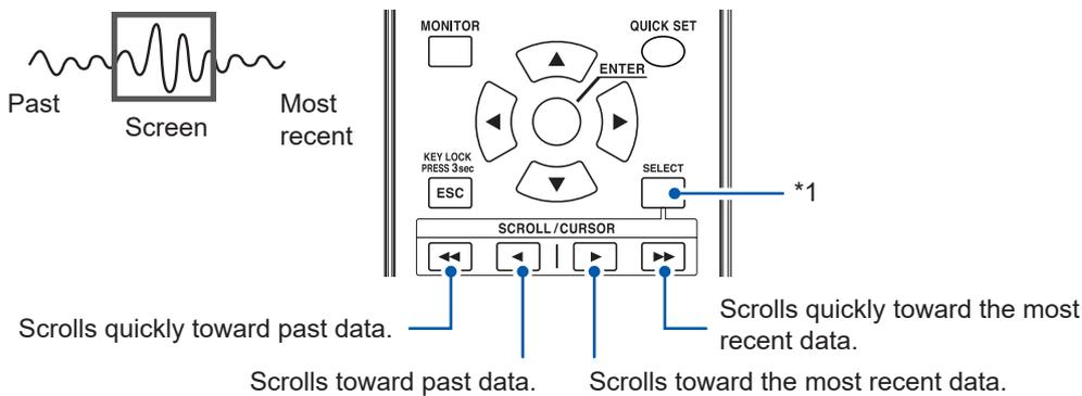
\*1: Switches the **SCROLL/CURSOR** keys function (waveform movement or A/B cursor movement). You can switch the amount of movement for the **SCROLL/CURSOR** keys by pressing and holding the **SELECT** key while you operate them.
