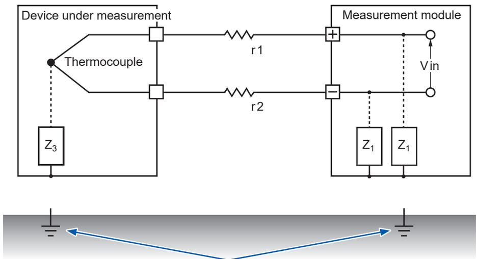
When measuring temperature with a thermocouple, the circuit will be susceptible to noise unless both the device under measurement and the measurement module have been grounded. This is not an issue when powering the measurement module with the battery, but ground the measurement module if using the AC Adapter.
