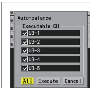
Auto-balancing can also be performed using the [Auto-balance] button on the top right of the channel list screen. Press the ENTER key to display the settings window.
