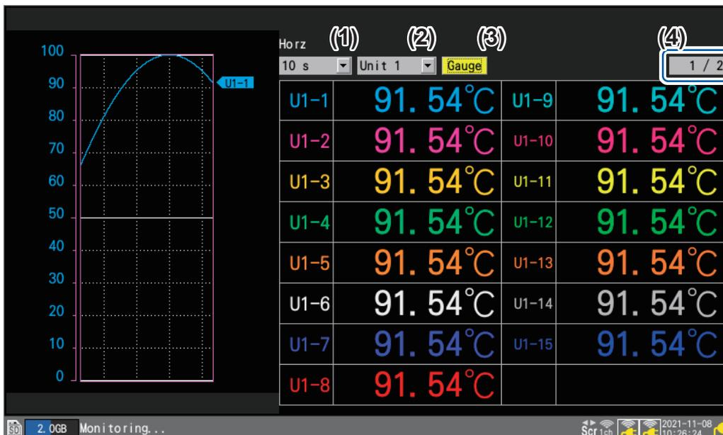
The monitor function will terminate when you change the screen display or start measurement.
