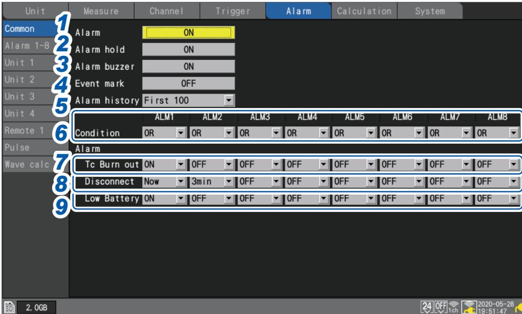
**1** Under **[Alarm]**, set the alarm function to **[ON]**.
