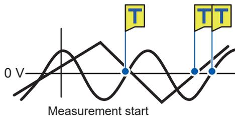
Activates the trigger when either one crosses 0 V from below to above.
