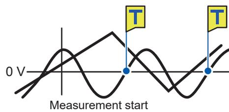
Activates the trigger when either one crosses 0 V from below to above while the other is exceeding 0 V.
