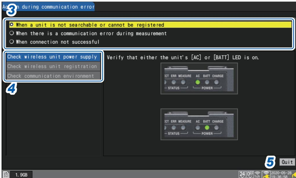
**3** Use the **Up Arrow** and **Down Arrow** keys to select the error type, and then press the **ENTER** key.
