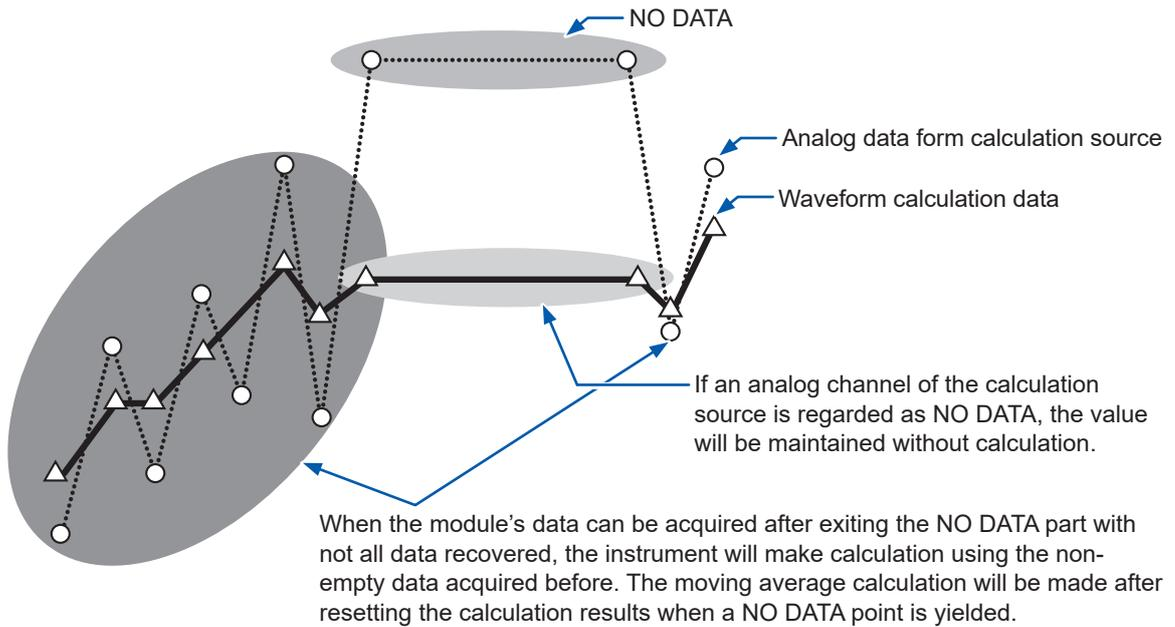
**Resetting waveform calculations**
