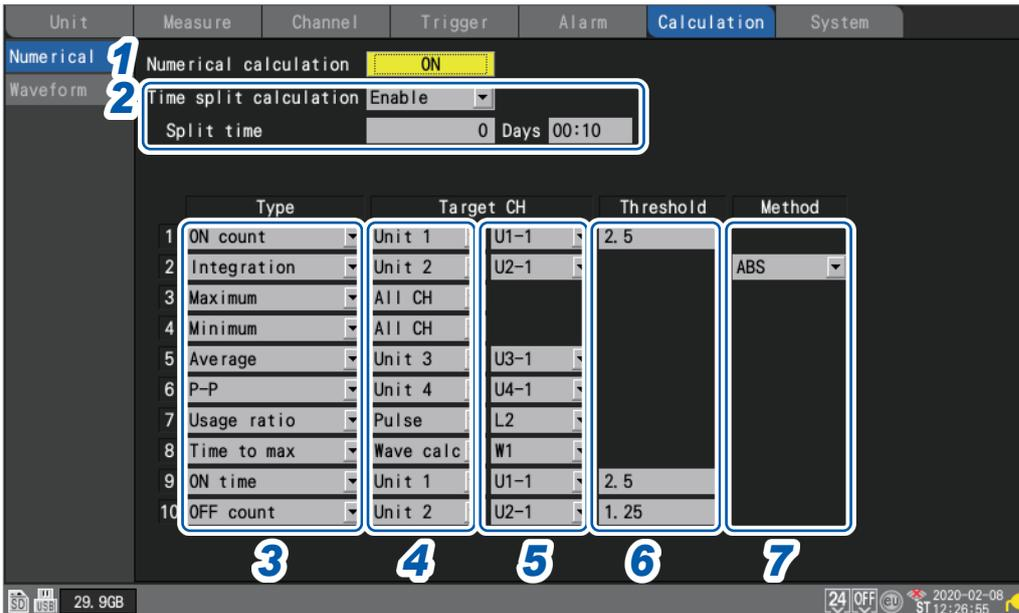
1 Under [Numerical calculation], set the numerical calculation function to [ON].
