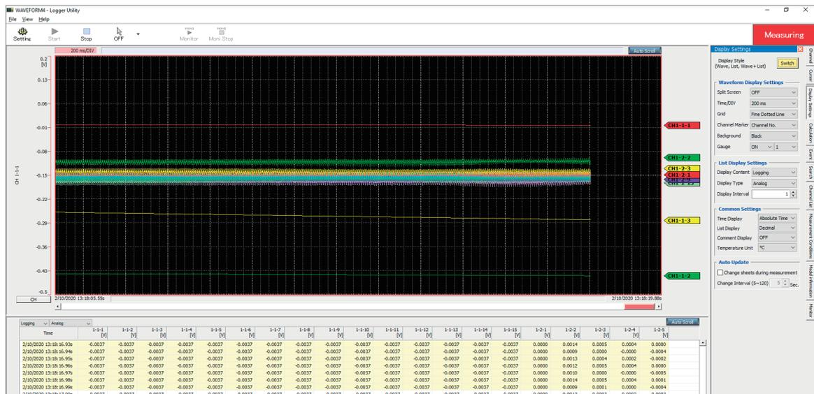
When a recording interval of between 1 ms and 5 ms is set, the system cannot acquire data in real-time.
