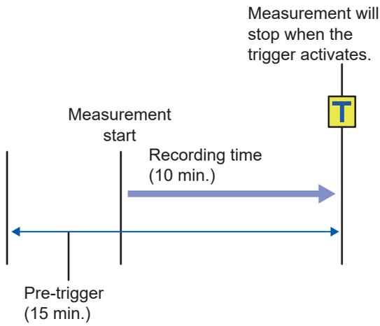
**If the recording time is longer than the pre-trigger**
