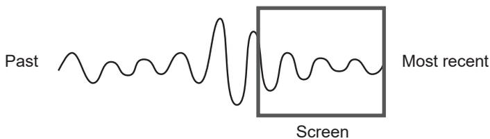
During measurement, press the **ENTER** key while **[Follow]** (on the bottom right of the screen) is selected or use the jump function to move to the end of the waveform.
