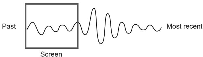
Use the jump function to move to the beginning of the waveform.
