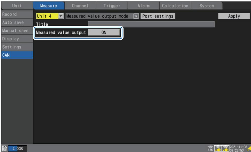
Settings controlling measured value output are configured with the CAN Editor. On the LR8450, you can select whether to output measured values overall.
