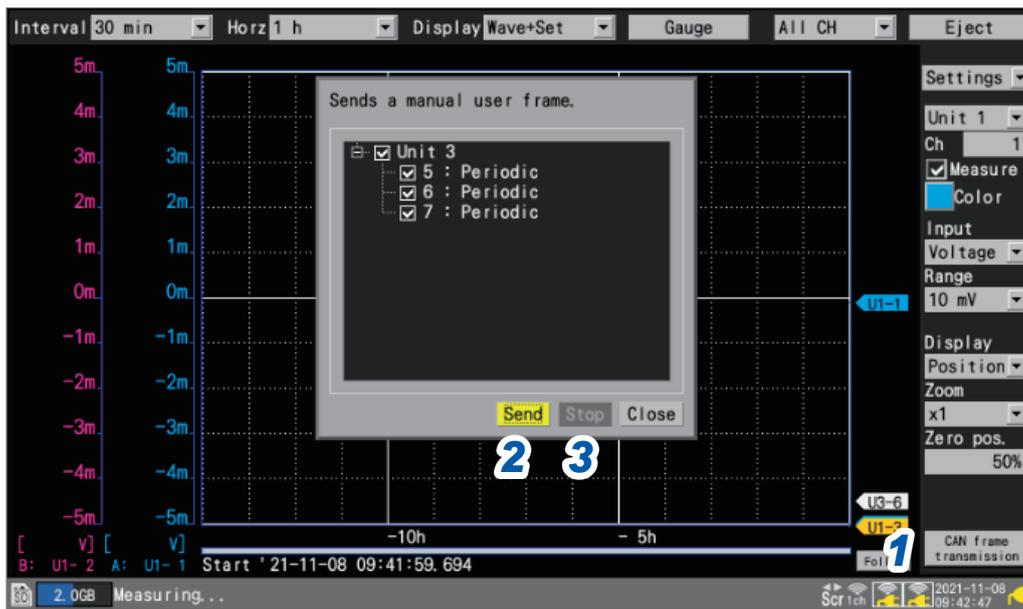
When measurement starts, **[CAN frame transmission]** will be displayed on the **[Wave+Set]** waveform screen.
