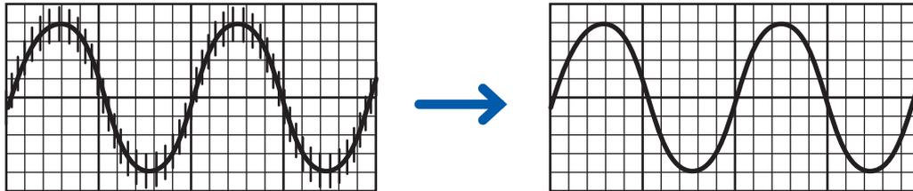
It is recommended to select the same frequency (50 Hz or 60 Hz) as the power supply frequency in the region where the instrument is being used.
