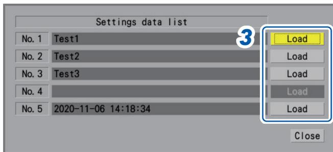
**3** Press the **ENTER** key with one of the **[Load]** buttons for **[No. 1]** to **[No. 5]** selected.
