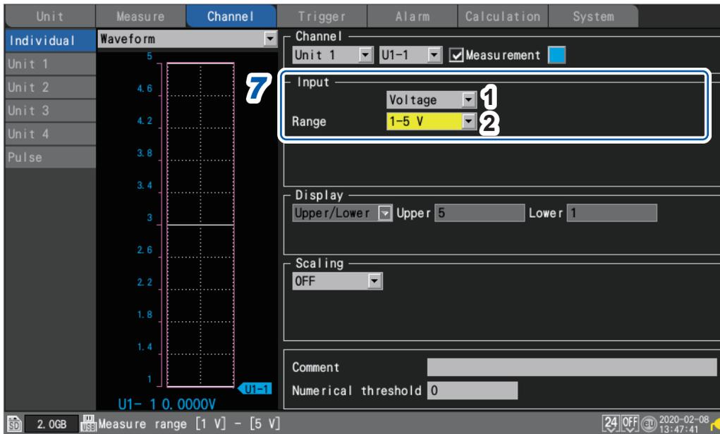
**7** Configure the settings as follows in the [Input] area for the channel being measured:
