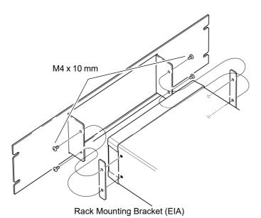
When mounting the unit in a rack, use, for example, a commercially available base for reinforcement
