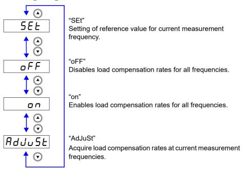
3. Press ENTER to confirm the load circuit compensation ON or OFF.
