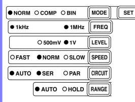
Using the keys on the operating panel, set the measurement conditions as shown at left.
