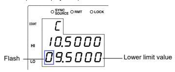
6. In the same way input the C lower limit value using the arrow keys or the numeric keypad.
