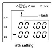
The reference value entered this time is not confirmed unless ENTER is pressed. The reference value used last time becomes valid.
