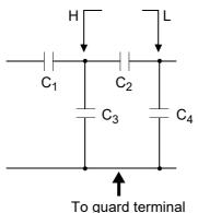
If you use a guard terminal as shown in the diagram, however, the current does not flow through capacitor  $C_4$  and the current that flows through capacitor  $C_3$  is absorbed by the guard terminal so that you can measure the capacitance of capacitor  $C_2$ .
