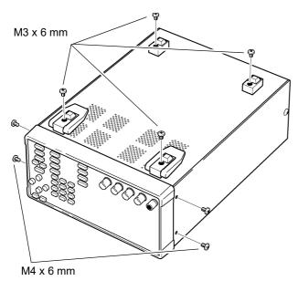
Remove the support legs from the bottom of the unit and screws from the side covers (4 screws at the front).
