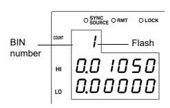
To make settings from an optional setting mode, press (a) (v) to select the setting mode while "1 to 13" is flashing, and then press (ENTER).
