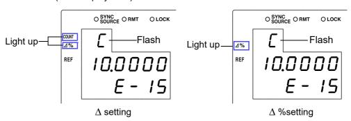
To make settings from an optional setting mode, press  $\P$  while "C" or "d"("q") is flashing to select the setting mode, then press  $\P$ . Setting modes: C upper limit and lower limit values  $\longleftrightarrow$  D (Q) reference value  $\longleftrightarrow$  D (Q) upper limit and lower limit values  $\longleftrightarrow$  C reference value...
