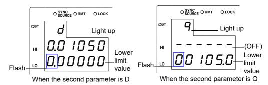
*12.* Enter the D (Q) lower limit value using the arrow keys or the numeric keypad.
