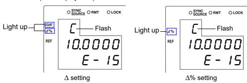
To make settings from an optional setting mode, press  $\bigcirc$  while "C" is flashing to select the setting mode, then press  $\bigcirc$  . Setting modes: C reference value BIN1 to 13 upper limit and lower limit values  $\longleftrightarrow$  D (Q) reference value  $\longleftrightarrow$  D (Q) upper limit and lower limit values  $\longleftrightarrow$  C reference value....
