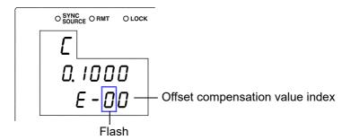
Input the C offset compensation value index with the arrow keys or the numeric keypad.
