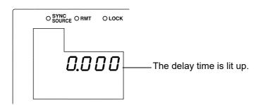
**3.** Press ♠ ♠ to enable or disable the trigger delay.
