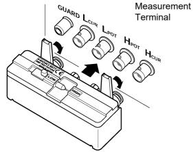
Position upwards the side of the device with the model number imprinted on it, plug directly into the measurement terminals and use the right-left levers to lock the connections.
