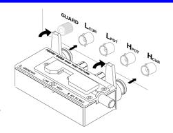
Connect the 9263 SMD Test Fixture to the measurement terminal.
