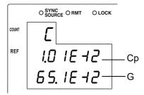
Pressing FREQ and LEVEL on the control panel and changing measurement conditions while the open circuit compensation values are being displayed will cause the compensation value relative to the set measurement conditions to be displayed.
