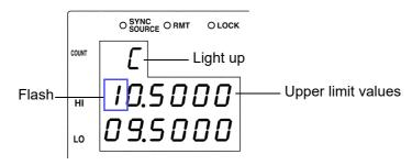
4. Input the C upper limit value using the arrow keys or the numeric keypad.
