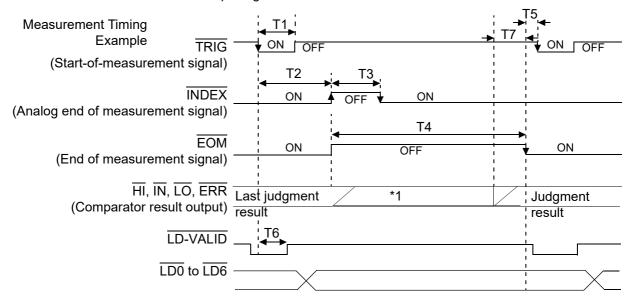
You can use a communication command to select whether the last judgement results for comparator measurement and BIN measurement are reset when analog measurement starts or held while analog measurement is performed and updated when analog measurement ends.
