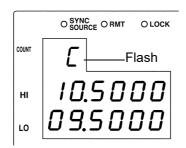
To make settings from an optional setting mode, press while "C" or "d"("q") is flashing to select the setting mode, then press ENTER.
