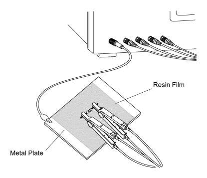
When measuring components on a metal plate, use, for example, resin film as insulation to ensure terminals and the like are not short-circuited.
