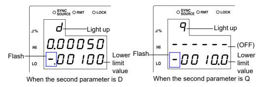
18. In the same way enter the D (Q) lower limit value using the arrow keys or the numeric keypad.
