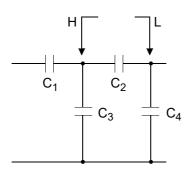
When measuring the capacitance of capacitor  $C_2$  as shown in the diagram, measure the parallel capacitance by adding up the value of the current that flows through capacitor  $C_2$  and the values of the current that flows through capacitors  $C_3$  and  $C_4$ , after the probes are connected to both sides of capacitor  $C_2$ .
