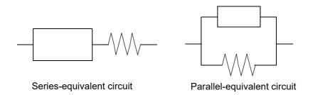
Normally, the series-equivalent circuit mode is used for a large capacitance (low-impedance components: approx. 100  $\Omega$  or less). While the parallel-equivalent circuit mode is used for a small capacitance (high-impedance components: approx. 10  $k\Omega$  or more). When you are not sure about selection of equivalent-circuit mode for the impedance such as between approx. 100  $\Omega$  to 10  $k\Omega$ ), please call the parts maker.
