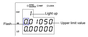
4. Use the numeric keypad or the arrow keys to enter an upper limit value for BIN1 and then press ENTER.
