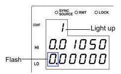
If \_\_\_\_\_\_ is not pressed, the BIN upper limit and lower limit values just entered will not be set.
