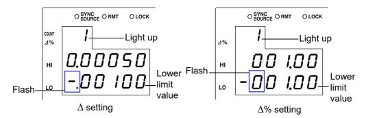
9. Enter the BIN1 lower limit value in the same way using the arrow keys or the numeric keypad.
