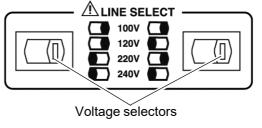
In the diagram, the voltage value is 100 V because both the left and right voltage selectors are set to the right side.
