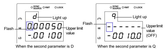
16. Enter the D (Q) upper limit value using the arrow keys or the numeric keypad.
