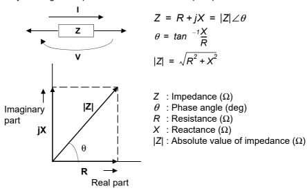
Furthermore, admittance Y that is the reciprocal of impedance Z can also be used depending on the characteristics of circuit components. As in the case of impedance Z, the following values can also be obtained from admittance Y by rotating the admittance Y around the complex plane
