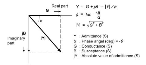
The unit calculates each of the elements using the following arithmetic expressions, based on a voltage V applied between terminals of the measurement sample, a current I that flows through the sample at that time, a phase angle  $\theta$  between voltage V and current I, and an angle speed  $\omega$  of the measurement frequency.
