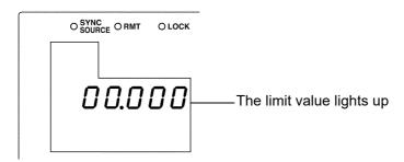
3. Press to enable or disable the Low C reject function.
