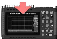
**START/STOP** : Lit the LED (green) at the left side of the key during measurement
