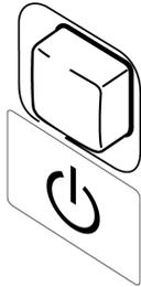
Press the power switch on the front of the instrument while it is in the standby state.
