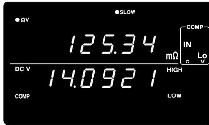
Resistance measurement and comparator display
