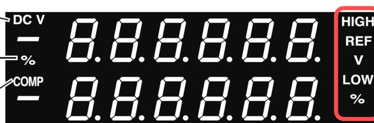
**HIGH, LOW** Indicates that absolute value comparator operation is enabled (while measuring), and also when setting.
