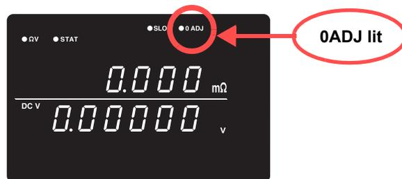
After measurement, the measured value of the compensation applied by the zero-adjust function is displayed.
