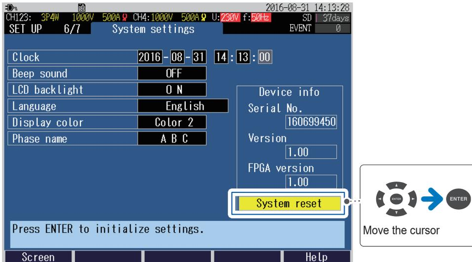
All settings other than the measurement frequency, clock, language, and communication settings (LAN and RS-232C) are initialized to their factory settings. The internal memory will not be cleared.
