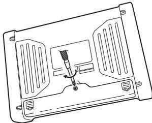
**4** Connect the plug of the Model Z1003 battery pack to the connector of the instrument. (Turn the 2 projection surfaces of the plug to the left and connect.)
