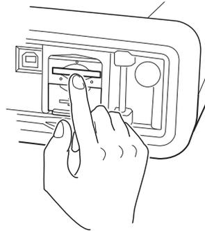
**3** Insert the SD memory card into the SD memory card slot on the computer.
