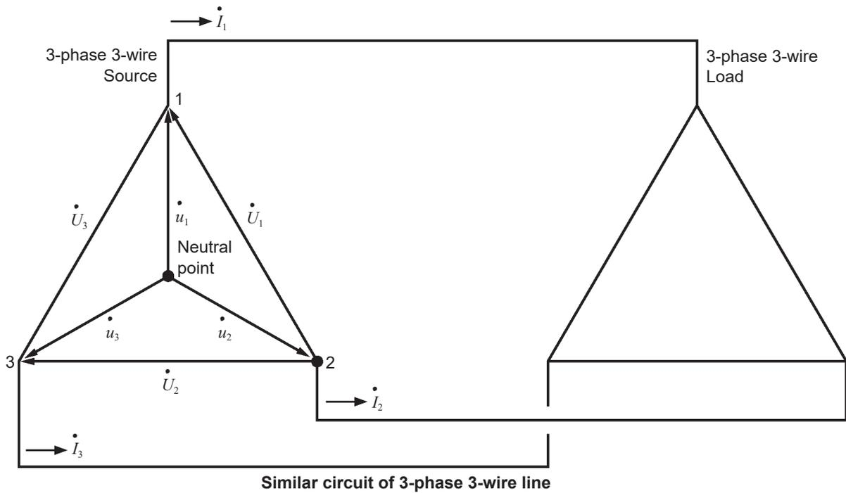
$\dot{U}_1, \dot{U}_2, \dot{U}_3$ : The vectors of line-to-line voltage
