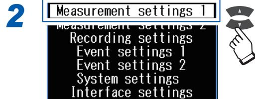
For the **SET UP, Interface Settings** screen, see “12 Communications (USB/LAN/RS-232C)” (p. 143) and “13 External I/O” (p. 173).
