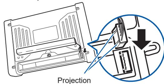
**5** Insert the battery pack in the direction that is indicated by the labeling on the battery pack.
