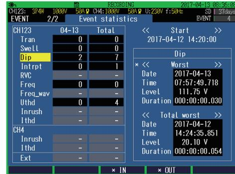
This screen is used to check the statistical results for each event type.
