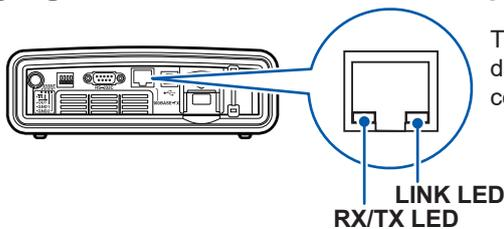
The RX/TX LED blinks during the transmission or reception of data. The LINK LED lights up, when the communication with the connected device is possible.
