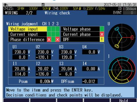
This screen is used to check whether the instrument has been connected properly.
