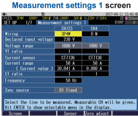
This screen is used to configure the wiring.
