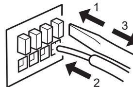
1. Press the terminal button down using a tool, such as a slotted screwdriver.
