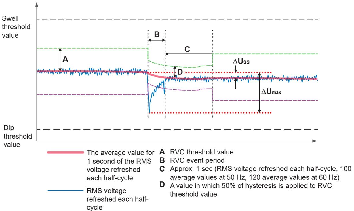
$\Delta U_{max}$ : Maximum absolute difference between the value for  $U_{rms(1/2)}$  and the average value for 1 second of the  $U_{rms(1/2)}$
