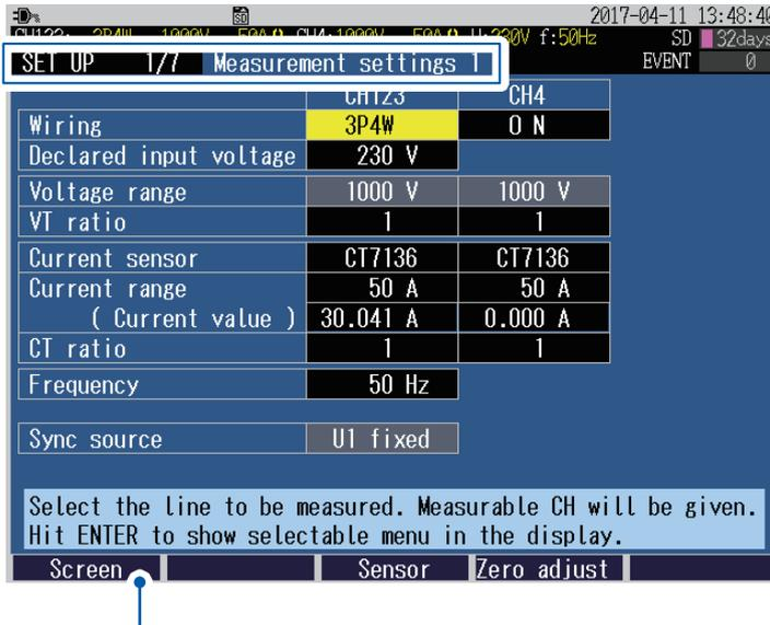
In addition to the **[SET UP]** key, you can switch to the **SET UP** screen from here also.
