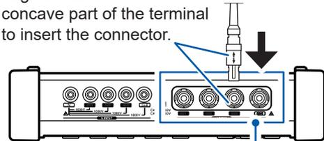
When disconnecting the current sensor, be sure to grip the part of the connector indicated by the arrows and pull it straight out.
