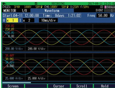
Voltage and current waveforms of CH1 to CH4 are displayed.
