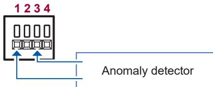
External devices are connected to **1** “Event input terminal (EVENT IN)” and **3** “Ground terminal for event input (non-isolated) (GND1).”
