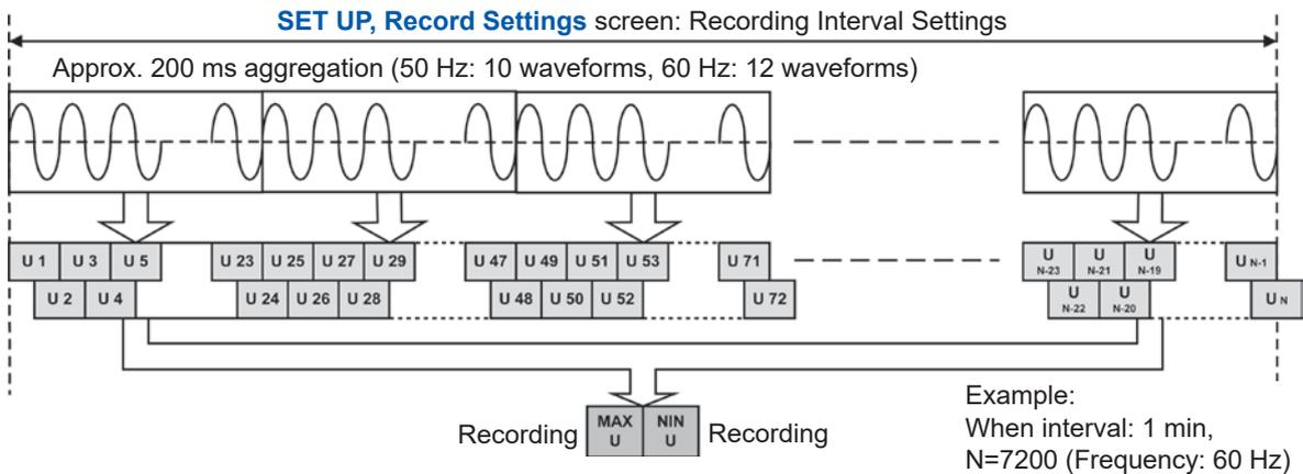
RMS voltage refreshed each half-cycle ( $U_{rms1/2}$ ) is calculated for one waveform shifted over half a wave.
