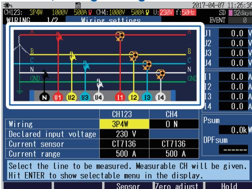
**2** Insert the connector of the current sensor while checking the channel on the screen.
