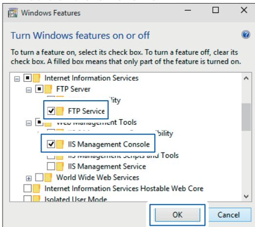
The FTP will be installed to the computer. After the installation, **inetpub** folder will be created under the root of the drive C.
