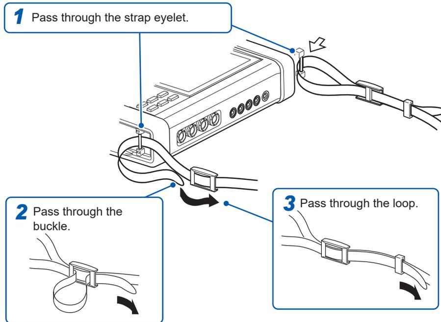
Tighten the straps securely to avoid loosening or twisting.
