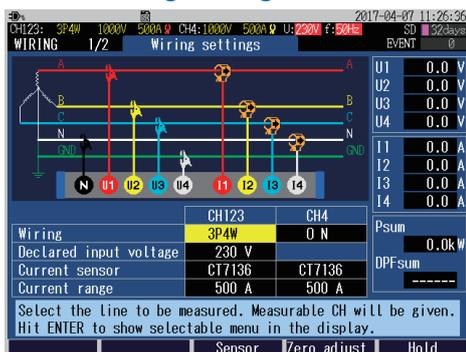
This screen is used to configure the wiring.
