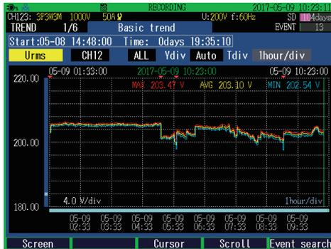
This screen is used to check fluctuation width of maximum, minimum and average values between recording intervals.
