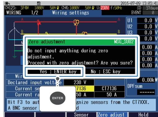
The DC components superimposing on voltage and current are adjusted to zero. It will take approximately 20 s.
