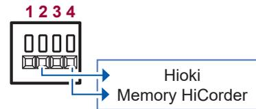
External devices are connected to **2** “External output terminal (EXTERNAL OUT)” and **4** “Ground terminal for external output (non-isolated) (GND2).”
