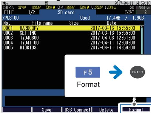
The SD memory card / the internal memory is formatted and the PQ3100 master folder is in it (p. 124).
