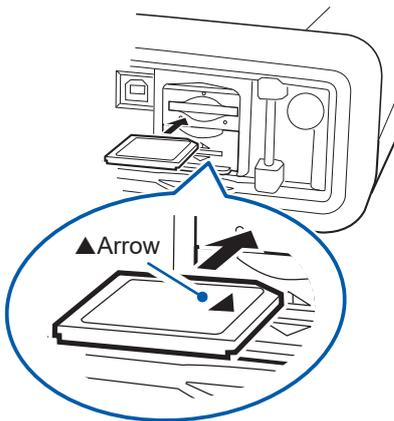
Insert the card horizontally. Inserting the SD memory card at an angle may cause the write-protect lock to engage, preventing data from being written to the card.
