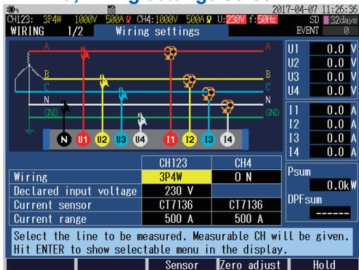
**3** Insert the voltage cord while checking the channel on the screen.
