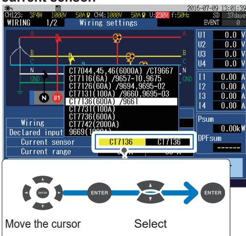
Example: Select **CT7136** for Model 9661 Clamp on Sensor
