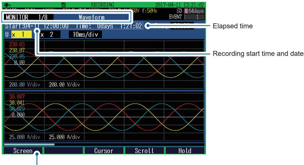
In addition to the **[MONITOR]** key, you can also switch to the **MONITOR** screen by using the **[F1] (Screen)** key.
