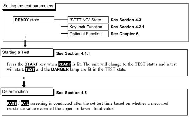
The flowchart below explains how a test is carried out.
