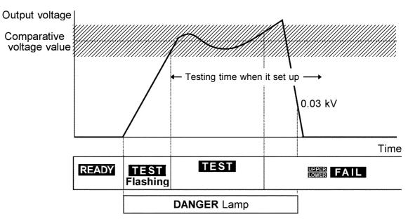
When the output-voltage deviates from the comparative-voltage range:
