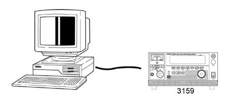
▲ CAUTION • Use a common ground for both the instrument and the computer. Using different ground circuits will result in apotential difference between the instrument's ground and the computer's ground. If the communicationscable is connected while such a potential difference exists, it mayresult in equipment malfunction or failure.
