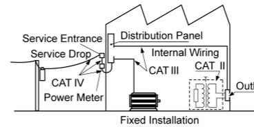
Using a measurement instrument in an environment designated with a higher-numbered category than that for which the instrument is rated could result in a severe accident, and must be carefully avoided. Use of a measurement instrument that is not CAT-rated in CAT II to CAT IV measurement applications could result in a severe accident, and must be carefully avoided.
