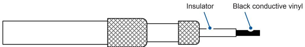
**8** Completely remove the conducting vinyl.
