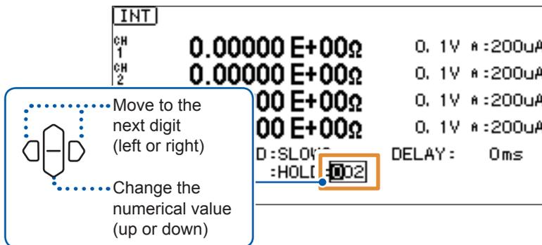
The numerical value can also be changed with the numeric keypad. See “Methods for changing numerical values” (p. 25).
