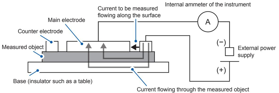
**(2) Measurement with the guard electrode**
