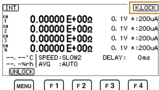
To unlock the key lock: hold the **MENU** key **[UNLOCK]** for more than 1 second.
