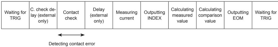
When contact check delay times of channels are different from each other
