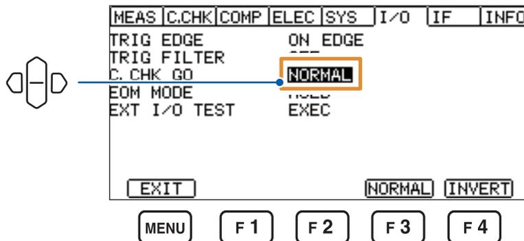
When the contact check is disabled, the instrument always gives fail judgments and thus outputs the Off signal.
