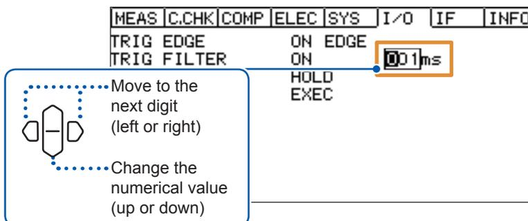
The numerical value can also be changed with the numeric keypad. See “Methods for changing numerical values” (p. 25).
