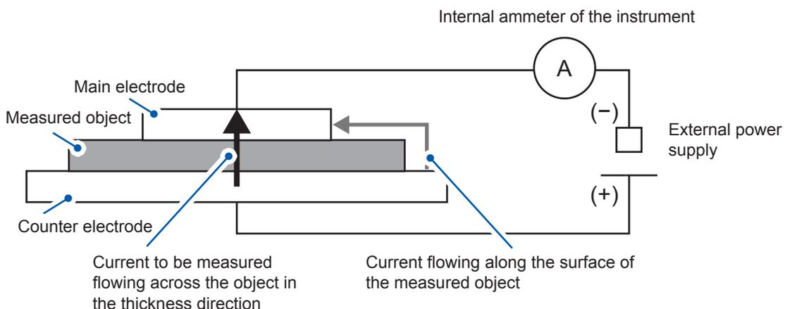
**(2) Measurement with the guard electrode**
