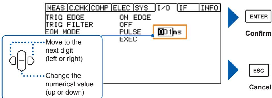
The numerical value can also be changed with the numeric keypad. See "Methods for changing numerical values" (p. 25).
