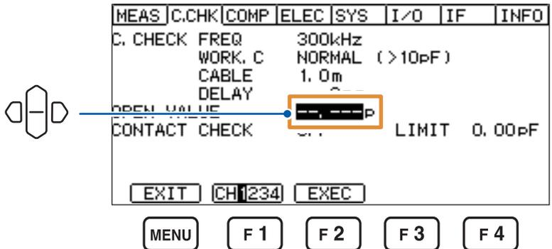
The open correction is executed, acquiring the correction value.
