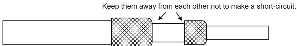
Take care not to short-circuit the shielding wire and the guard wire with each other.
