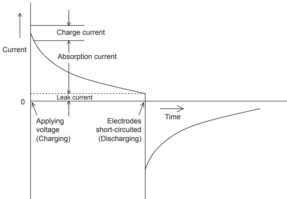
Figure 2 Dielectric Absorption
