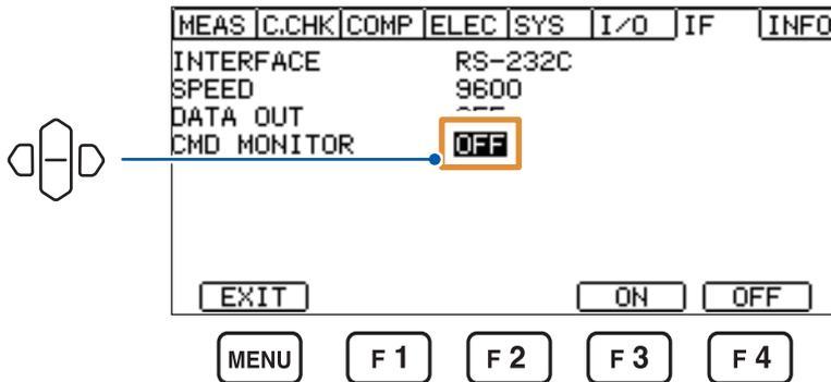
The communication monitor is displayed on the measurement screen when communication starts.
