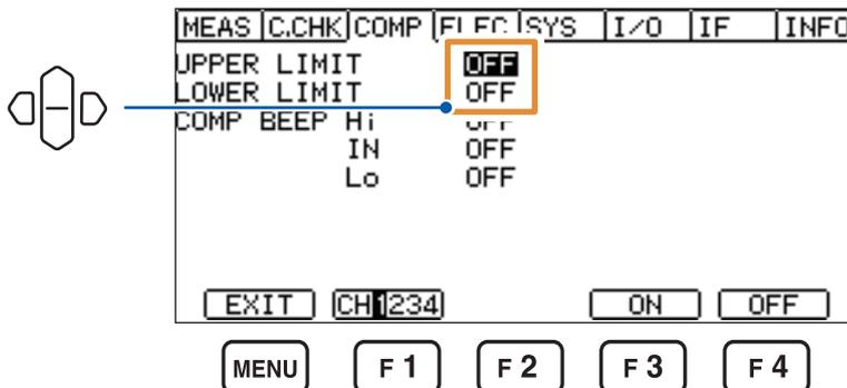
**2** If the upper limit and lower limit settings are set to [ON], set the numerical value.
