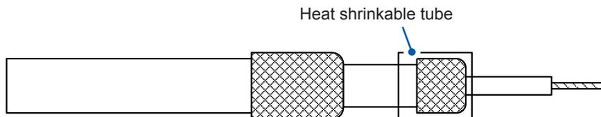
**10** Cover the shielding wire with a heat shrinkable tube and make it shrink.
