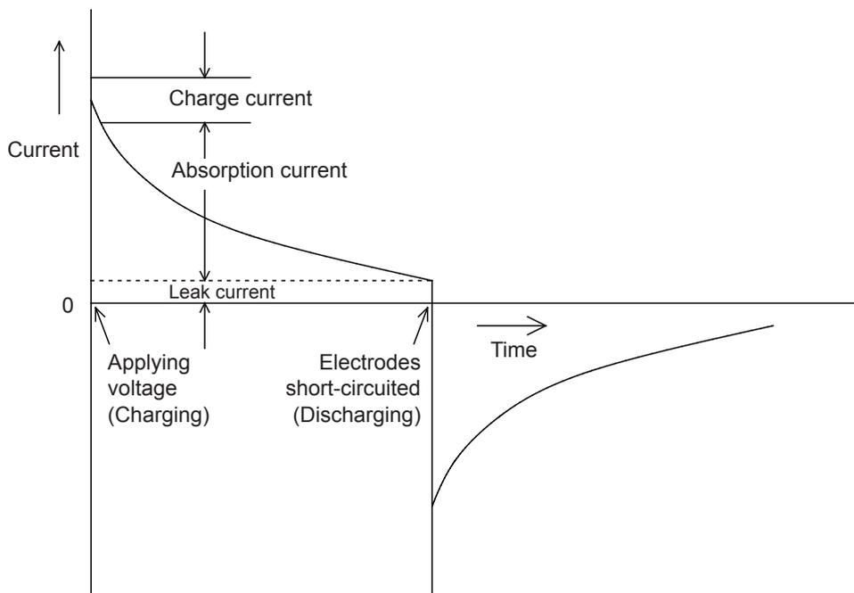
Figure 2 Dielectric Absorption
