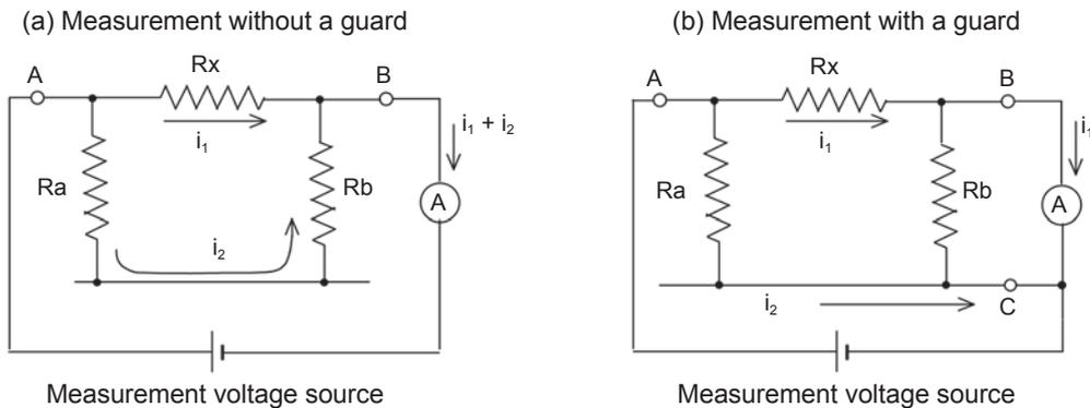
The figures “Example of use” and “Principles of the guard” explain the effectiveness of the guard. Considering how the current flows from Terminal A to Terminal B in the “Example of use,” 2 flow channels are found.
