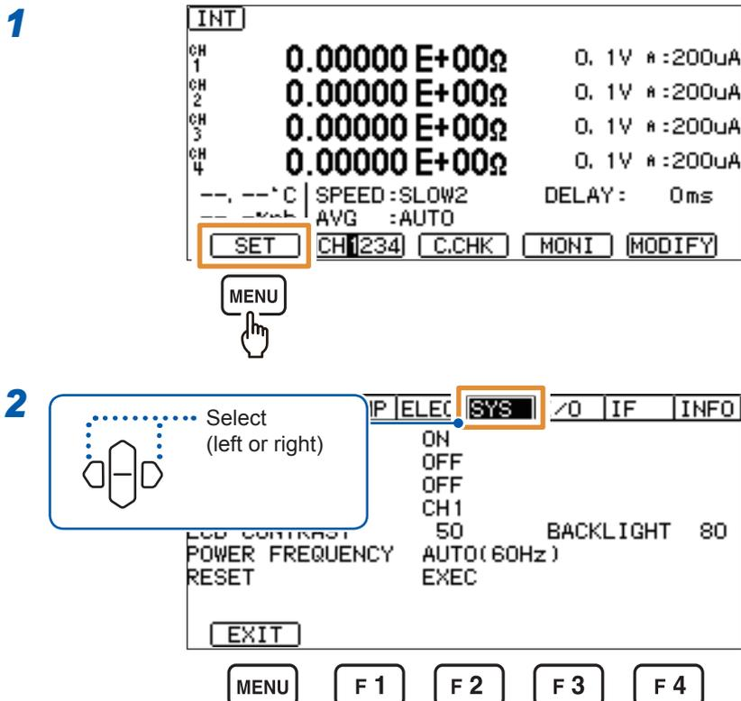
In this manual, the procedure to display the settings screen is described as follows:
