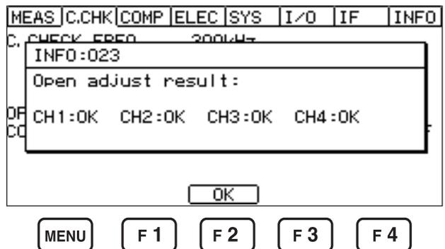
A short-circuit between the INPUT and OUTPUT terminals will cause the fixture capacitance open correction to fail, displaying a result “NG.” Check a short-circuit between the terminals.
