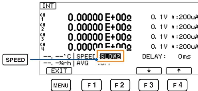
The measurement speed changes every time the F3 key [↓] is pressed in the following order: FAST, FAST2, MED, SLOW, and SLOW2.
