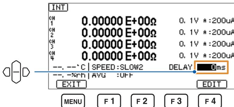
Pressing the **F4** key [**EDIT**] enables the numerical value to be changed in increments of 1 ms.
