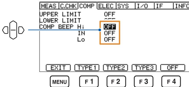
Selecting [TYPE1], [TYPE2], or [TYPE3] sounds the buzzer in a specific tone for confirmation.
