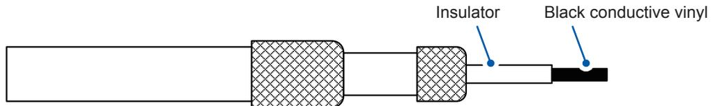
**8 Completely remove the conducting vinyl.**
