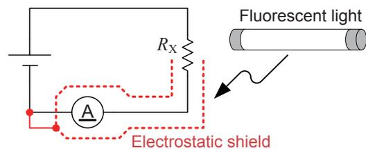
Figure 1 Electrostatic shield close to high-voltage wiring
