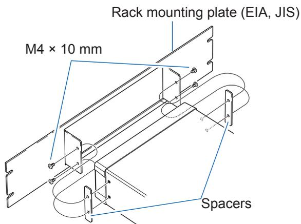
**2** Install the spacers on both sides of the instrument, secure the rack mounting plate with the M4 × 10 screws.
