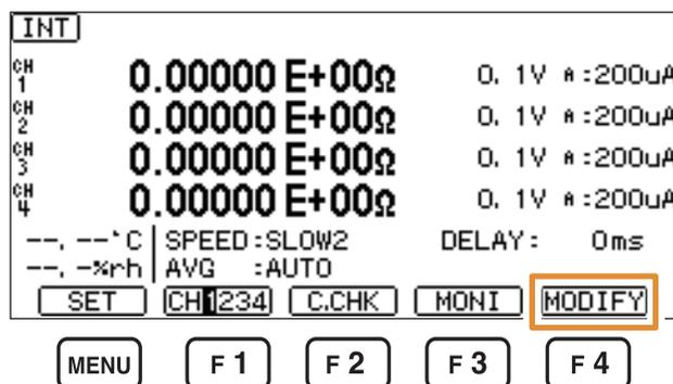
Pressing the **ESC** key cancels the changes of the measurement conditions.
