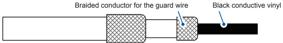
**6 Completely remove the conducting vinyl.**
