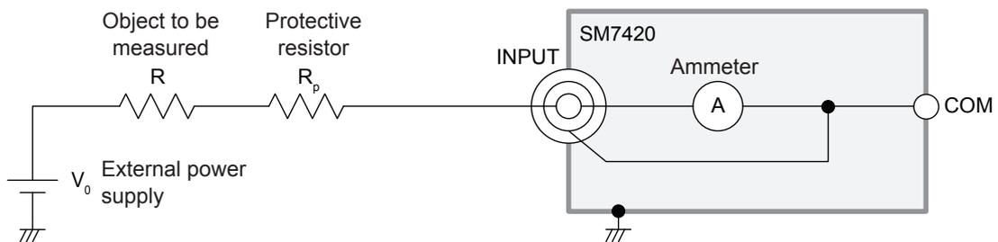
When using the external power supply, insert a protective resistor so that a current flowing through the instrument is reduced to the rated current or less even if the terminals of the object to be measured are short-circuited with each other.
