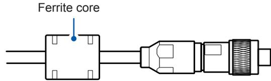
Figure 3 Ferrite core
