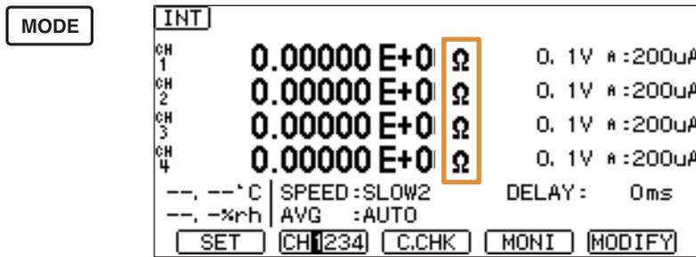
The instrument displays values that include the input resistance of 1 kΩ (±10%).
