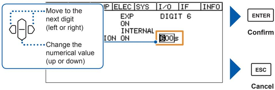
The numerical value can also be changed with the numeric keypad. See “Methods for changing numerical values” (p. 25).
