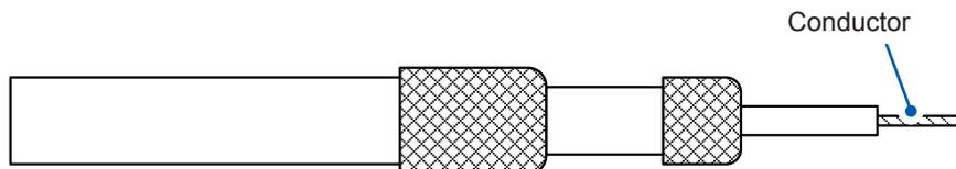
**9** Cover the guard wire with a heat shrinkable tube and make it shrink.
