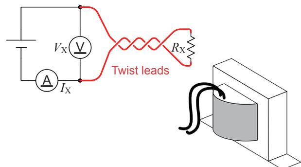
Figure 2 Twist leads close to a high-current line
