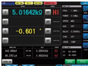
The LCR function allows you to measure the passive elements of capacitors and coils with a single measurement condition. This is suitable to make pass/fail judgments and classification on production lines.
