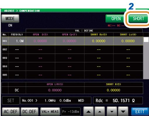
**1** Connect the standard unit for short to the test sample connection terminal.
