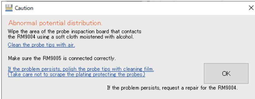
A description of how to resolve the FAIL result is shown in the window. Please refer to this information when performing probe maintenance.
