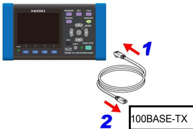
When connecting the instrument directly to a computer
