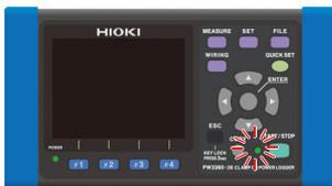
The recording LED flashing
