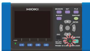
The recording LED flashing
