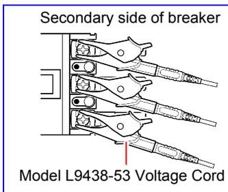
Securely clip the cords to the metallic part of the screw or wiring bar on the secondary side of the circuit breaker.
