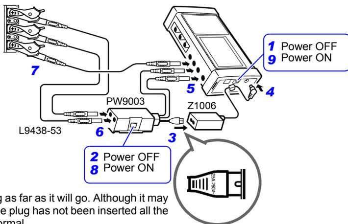
Insert the plug as far as it will go. Although it may appear that the plug has not been inserted all the way, this is normal.
