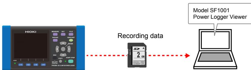
To access data, either load it from the SD memory card on which it was saved using a computer with an SD memory card reader, or use a USB cable to copy data from the SD memory card or internal memory to the computer.
