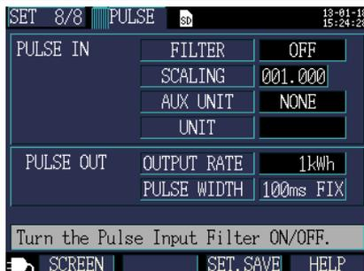
Filter ON (mechanical contact use):
