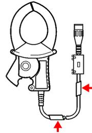
**2 Group together multiple clamp sensor cables with spiral tubes.**
