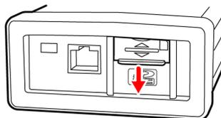
**3** Disengage the SD memory card's write-protect lock.
