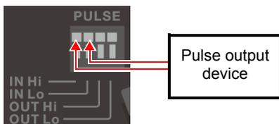
Input a pulse signal from an external source. After configuring scaling (coefficient), sub-unit, and unit (five byte characters) settings, you can convert and measure an input pulse signal. After recording and measurement are started, pulse input values are saved for each save interval.
