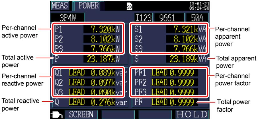
When using the 3-phase/3-wire/2-wattmeter method (3P3W2M), the active power, reactive power, apparent power, and power factor for each channel are obtained by means of a two-wattmeter calculation process and do not have physical significance. However, values for individual channels can serve as reference data when checking the connection.
