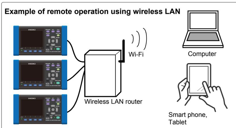
**NOTE** To connect several units of the PW3360 to a wireless LAN router
