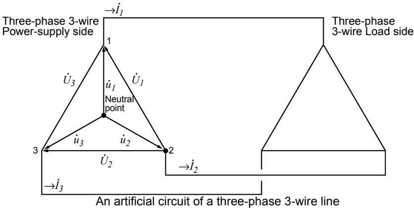
$\vec{U}_1, \vec{U}_2, \vec{U}_3$  : The vectors of line-to-line voltage
