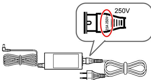
Connect the Z1006 AC Adapter to the instrument and plug it into an outlet as follows:
