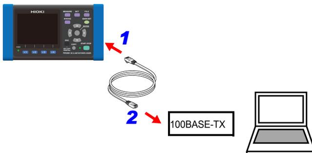
**NOTE** Since the instrument provides functionality for automatically detecting whether a straight or cross cable is being used, a straight cable may also be used. If you are unable to establish communications with the computer, try a cross conversion cable (9642 accessory).
