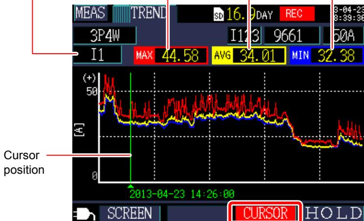
The cursor keys can be used to move the cursor. When the cursor is selected, time-series display updates stop.
