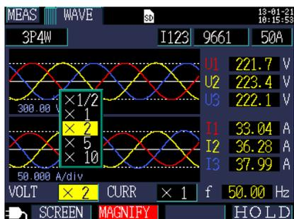
**3** Select the desired zoom factor with the cursor's **▲**/**▼** keys and press the **[ENTER]** key.
