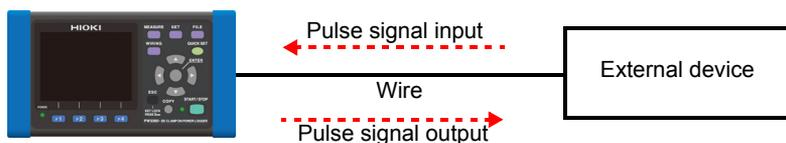
**1** Wire the instrument to an external device. (p. 172)
