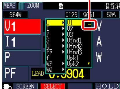
**3** Select the desired parameter with the cursor keys and accept the new setting with the
