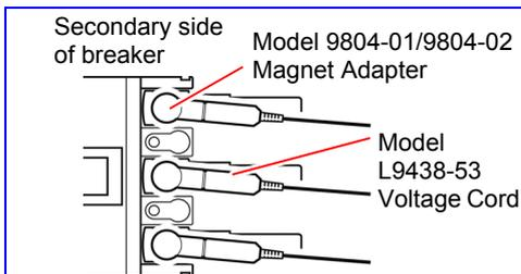
Connect the magnetic part of the 9804-01 or 9804-02 tip to the screws on the secondary side of the breaker.
