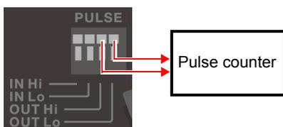
A pulse signal is output each time active energy consumption (WP+) exceeds the pulse output rate during recording and measurement. The output rate can be set from 1 Wh to 1,000 kWh.
